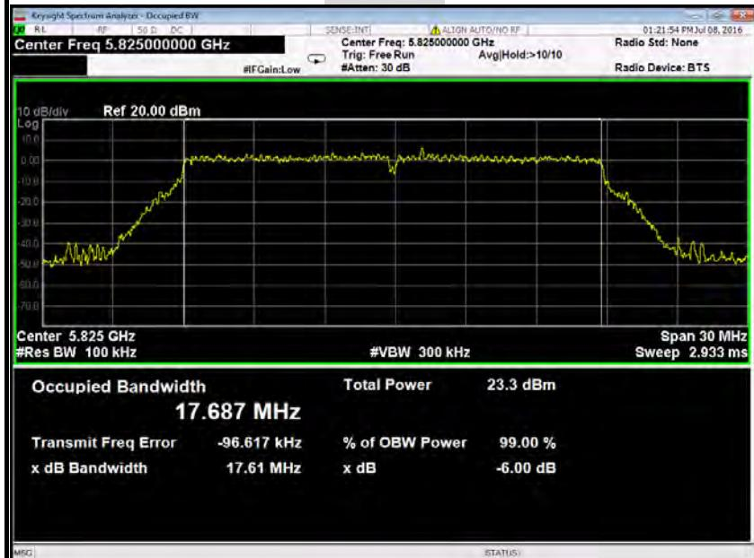
**IEEE 802.11n HT 20 MHz mode / 5745 ~ 5825MHz****6dB Bandwidth (CH Low)****Antenna 1**
