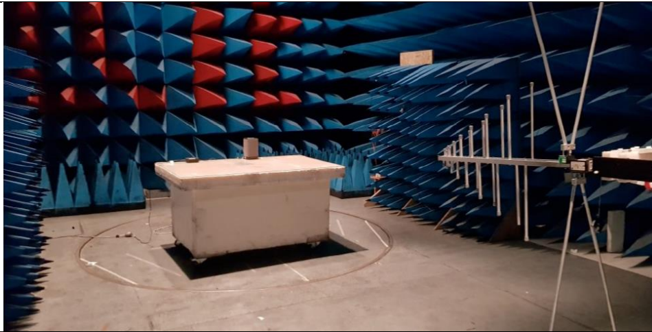
MEASUREMENT OF RADIATED DISTURBANCES ABOVE 1 GHz
