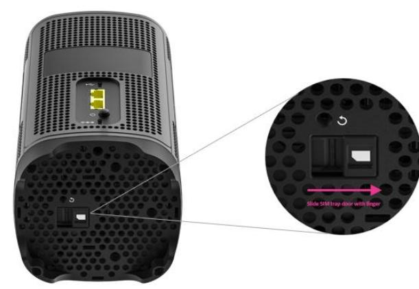
3. The SIM card socket supports push-in and push-out installation
