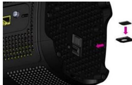
10. Be sure the SIM tray clicks into place to ensure that it is properly installed
