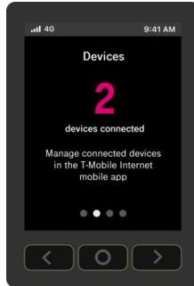
The Devices LCD screen on the front of the gateway shows the number of devices currently connected to the network by way of either Wi-Fi or Ethernet.
