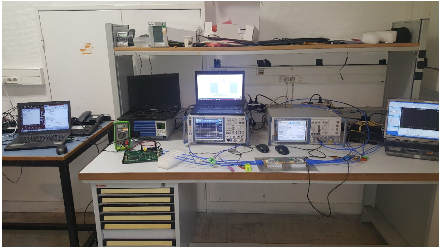
Photograph for Channel Availability Check Time & DFS Detection Threshold
