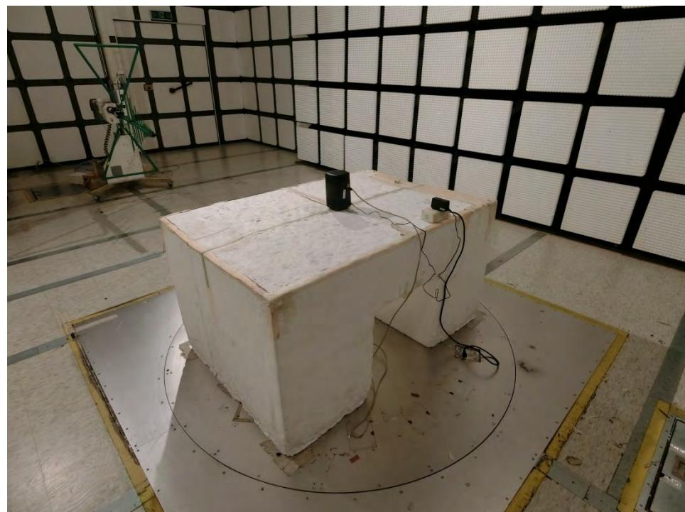
**Test Configuration: Above 1GHz****FRONT VIEW**
