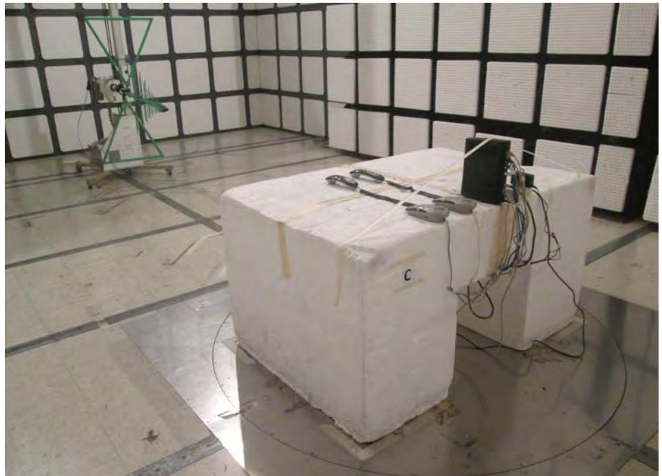
**Test Configuration: Above 1GHz****FRONT VIEW**
