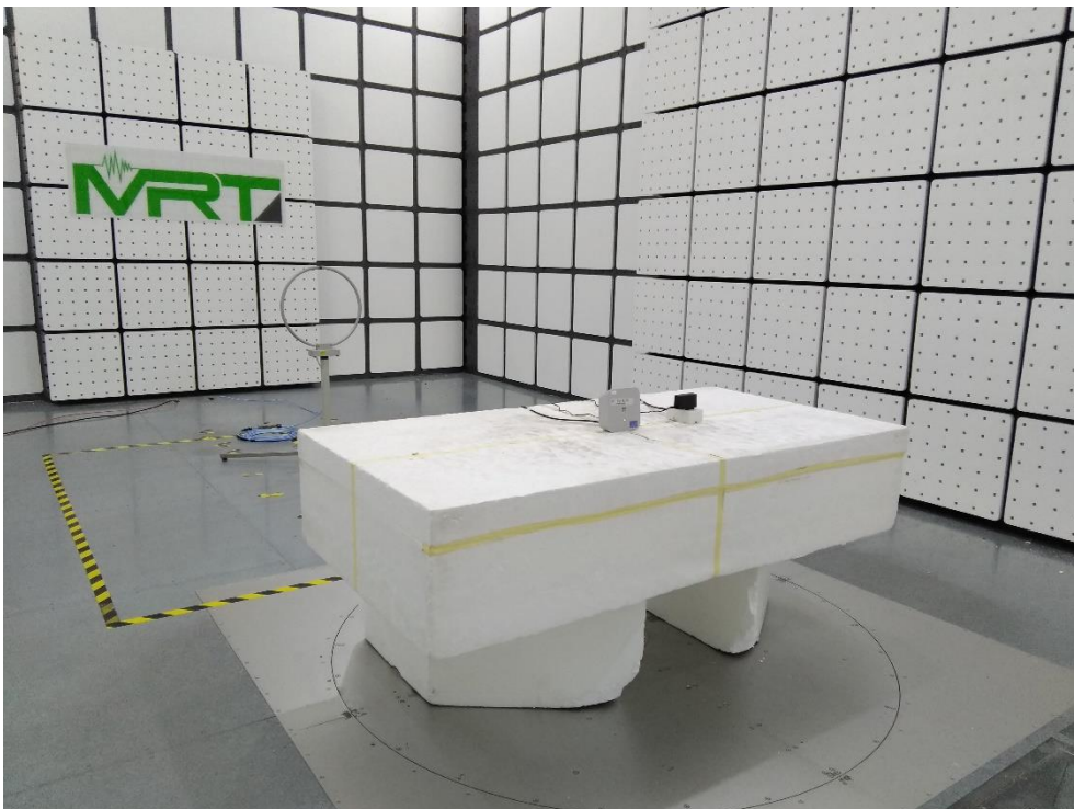
Description: Radiated Emission Test Setup for 9kHz~30MHz
