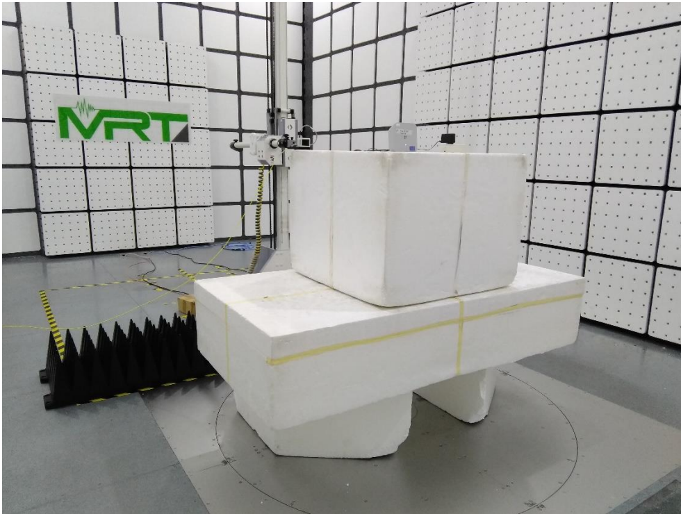
Description: Radiated Emission Test Setup for 9kHz~30MHz
