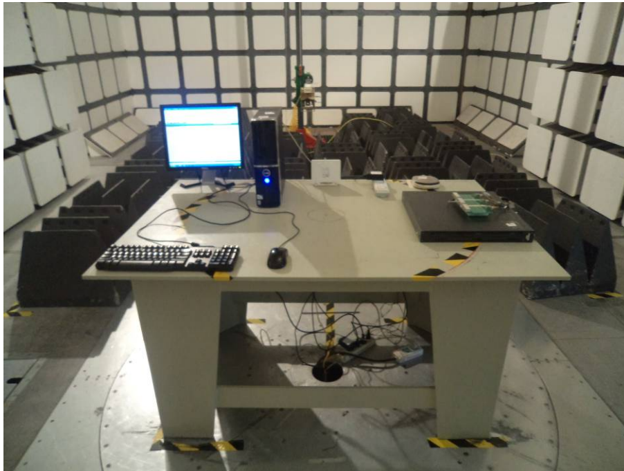
Spurious Radiated Emissions – Front View (Above 1 GHz)
