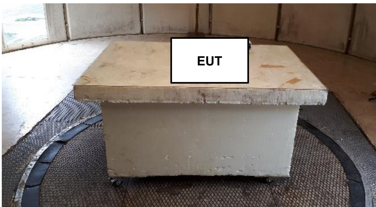
Test Set up for radiated measurement in open area test site
