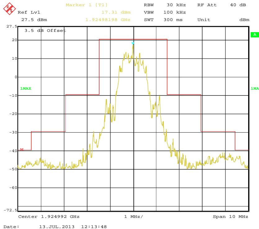
**Channel 0 (Unwanted Emission inside the Sub-band)**
