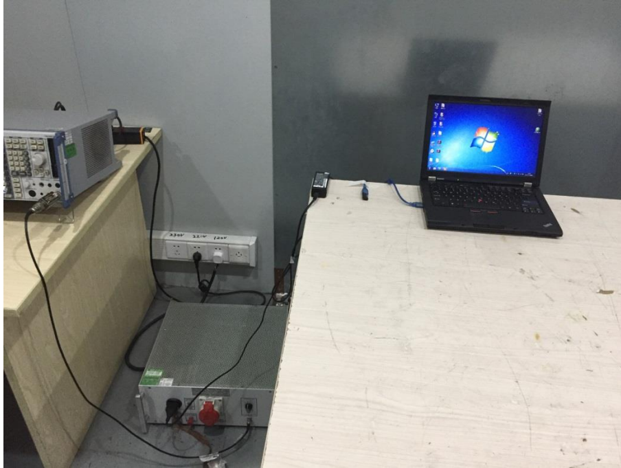
Radiation Emission Test Setup (Below 30MHz)
