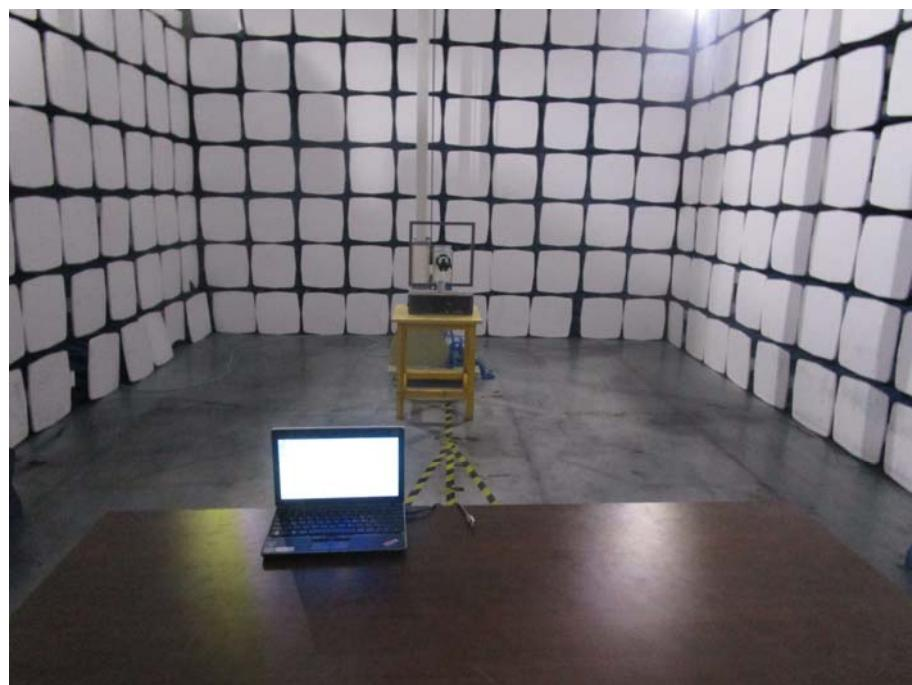
**Radiation Emission Test Setup (30MHz to 1GHz)**
