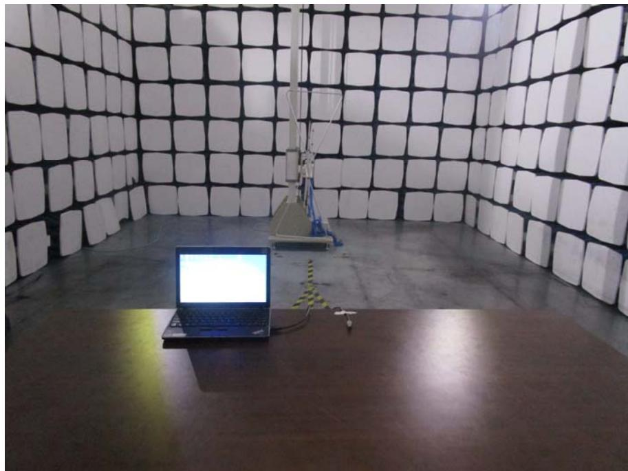
**Radiation Emission Test Setup (Above 1GHz)**
