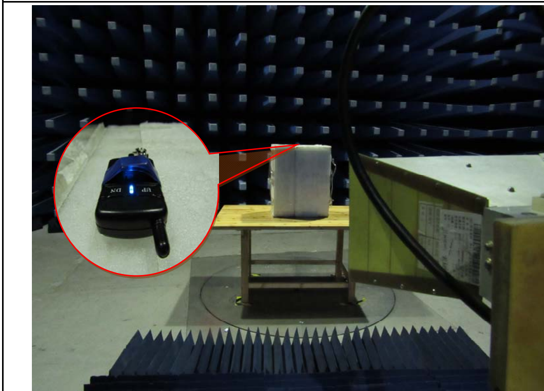
Radiated Spurious Emissions Test Setup Above 1GHz
