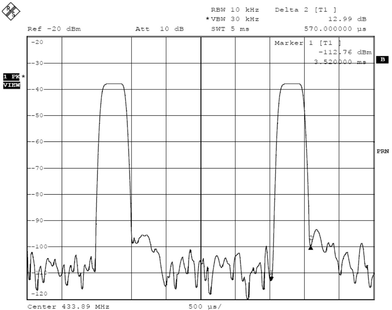
The graph shows the duration of 'on' signal. From marker 1 to marker 2, duration is 0.57ms.
