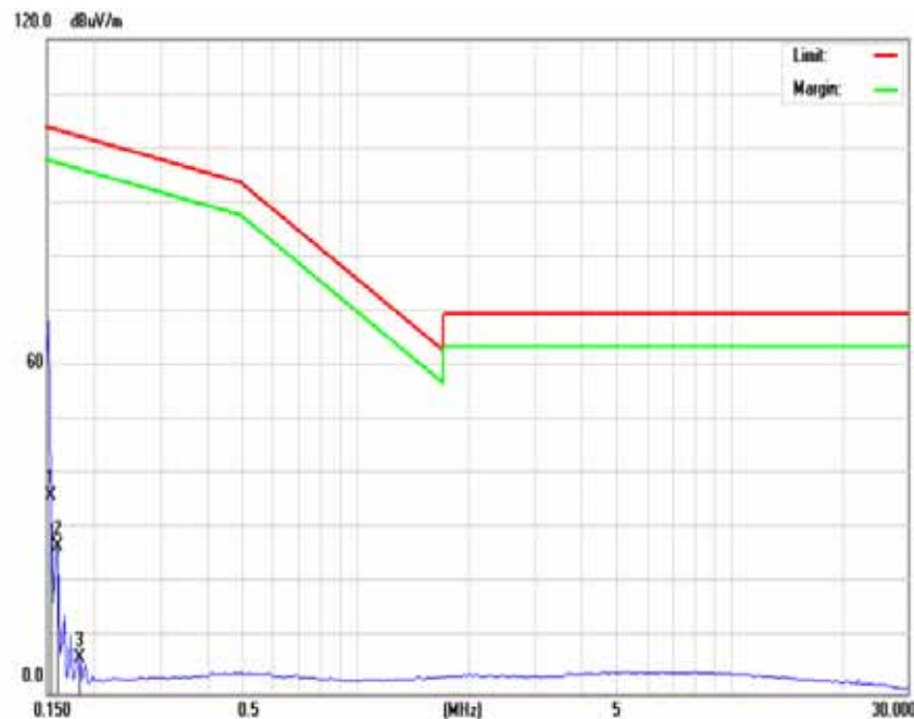
Field strength Emission Plot (Peak, Max Hold Mode 0.15MHz-30MHz)
