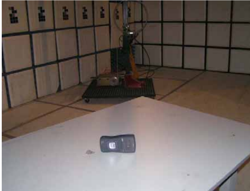
Low Frequency Radiated Emission Test Set-Up #1
