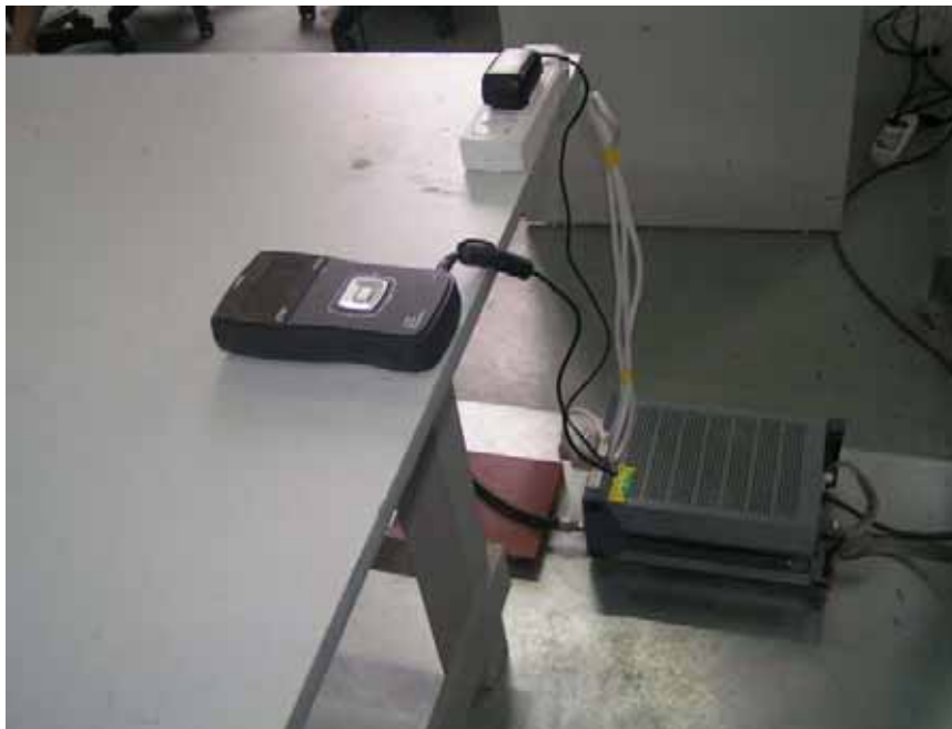
Conducted Emission Test Set-up - Side View
