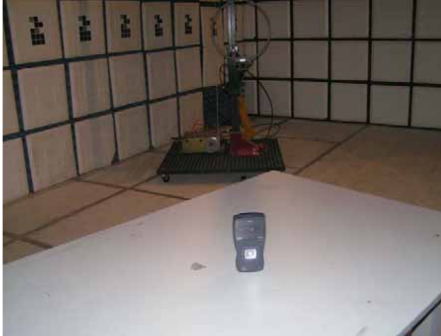
Low Frequency Radiated Emission Test Set-Up #1
