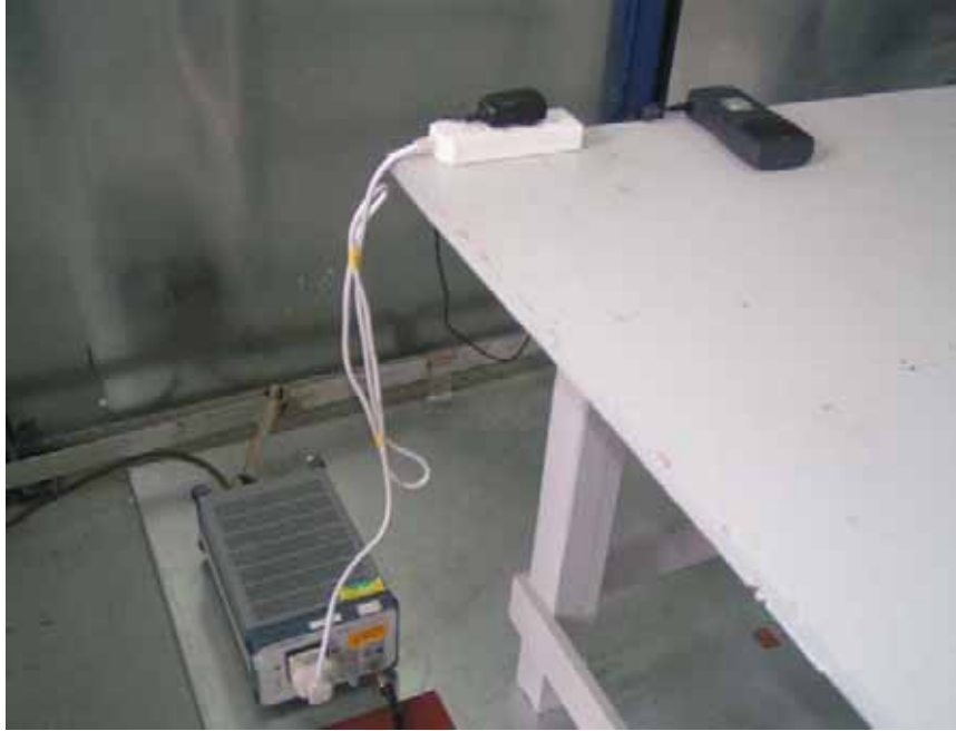
Conducted Emission Test Set-up - Front View
