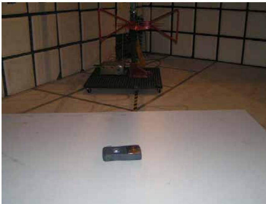
High Frequency Radiated Emission Test Set-Up
