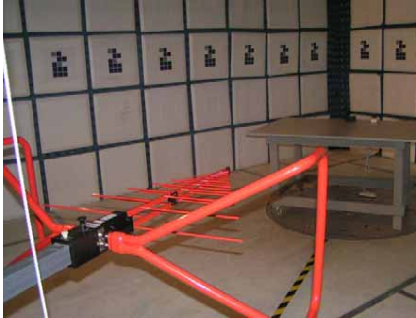
Radiated Emission Test Set-Up – Front View
