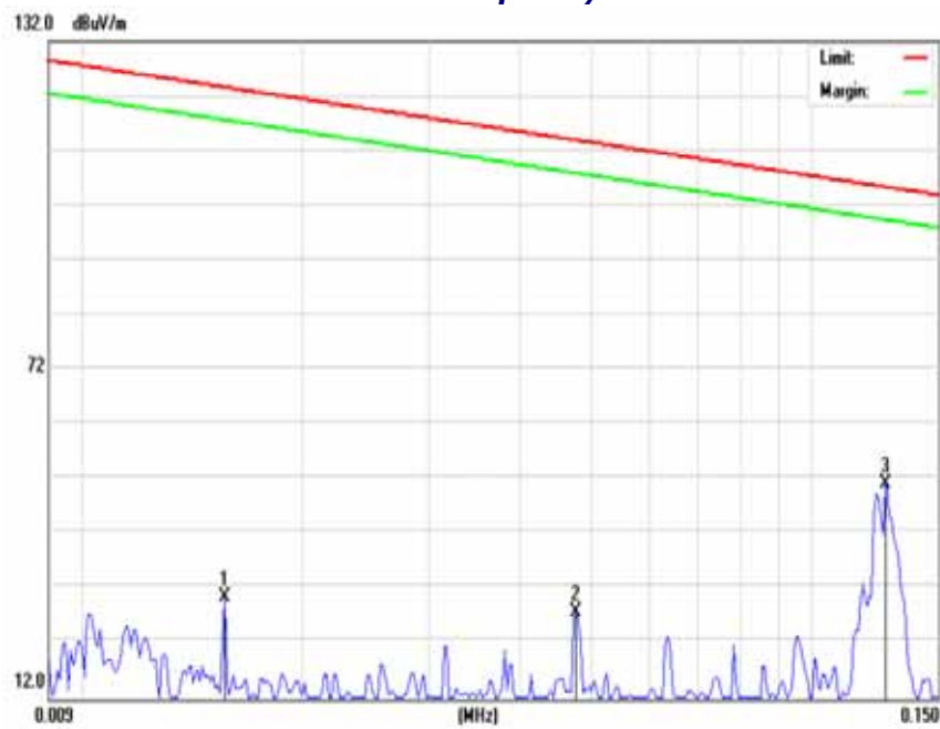
Field strength Emission Plot (Peak, Max Hold Mode 9kHz-0.15MHz)
