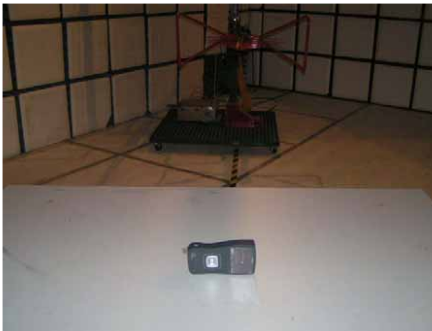
High Frequency Radiated Emission Test Set-Up
