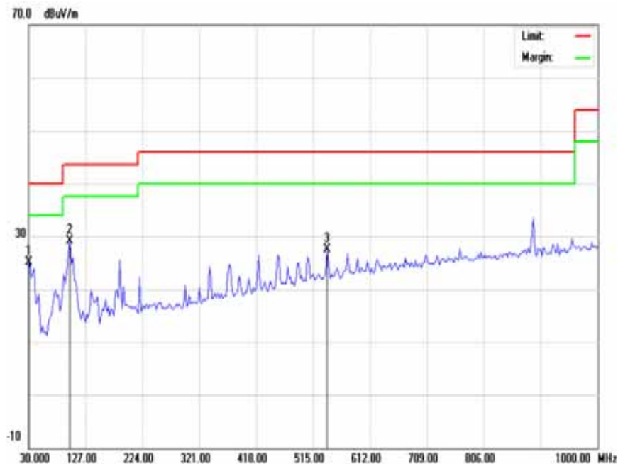
Field strength Emission Plot (Peak, Max Hold Mode Vertical)
