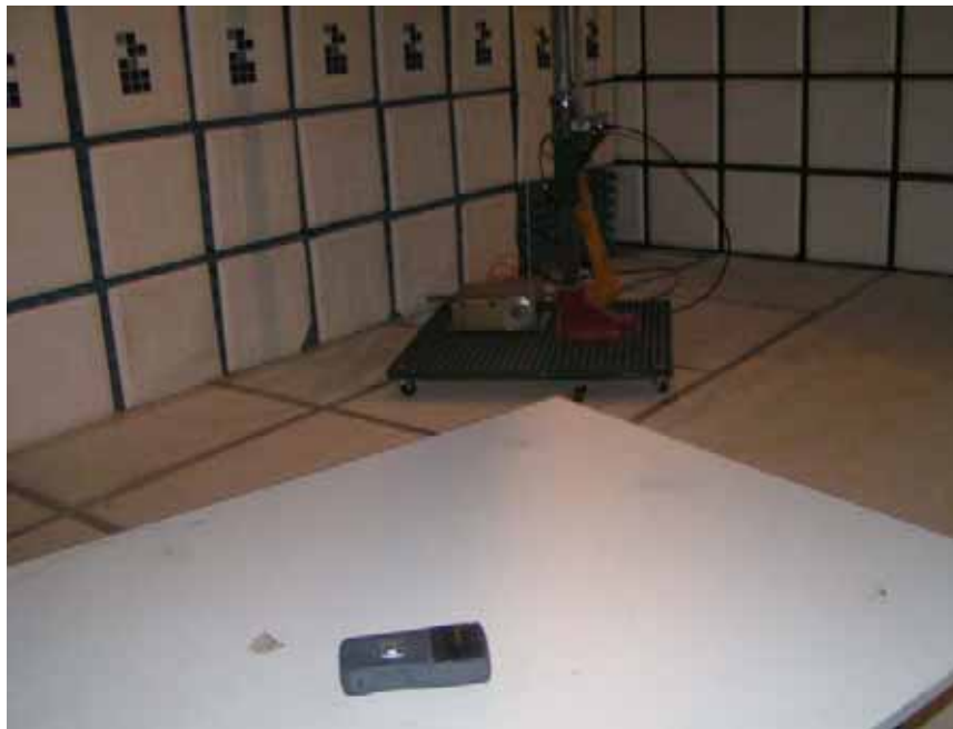
Low Frequency Radiated Emission Test Set-Up #2
