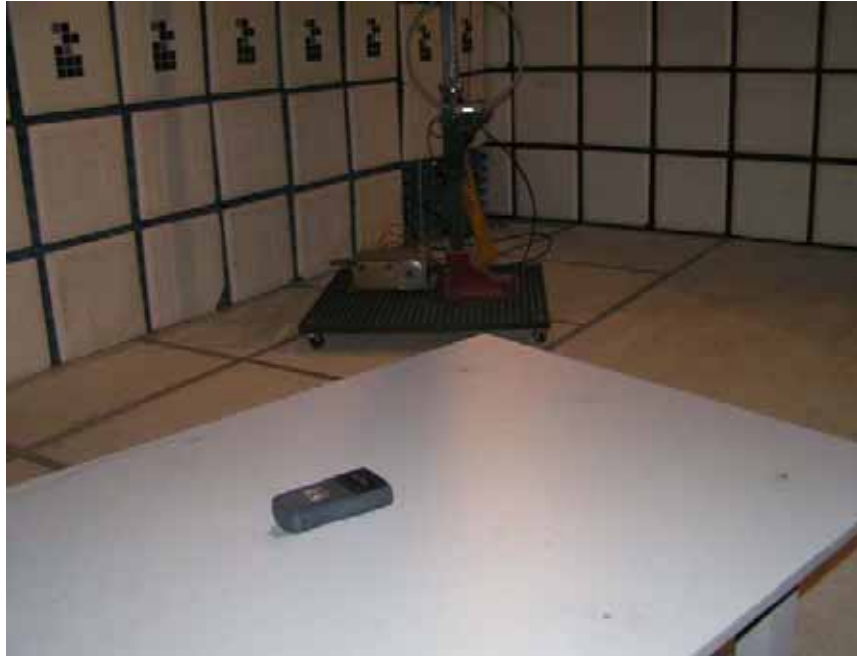
Low Frequency Radiated Emission Test Set-Up #1
