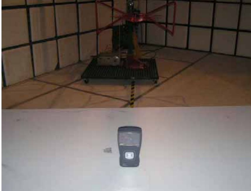
High Frequency Radiated Emission Test Set-Up
