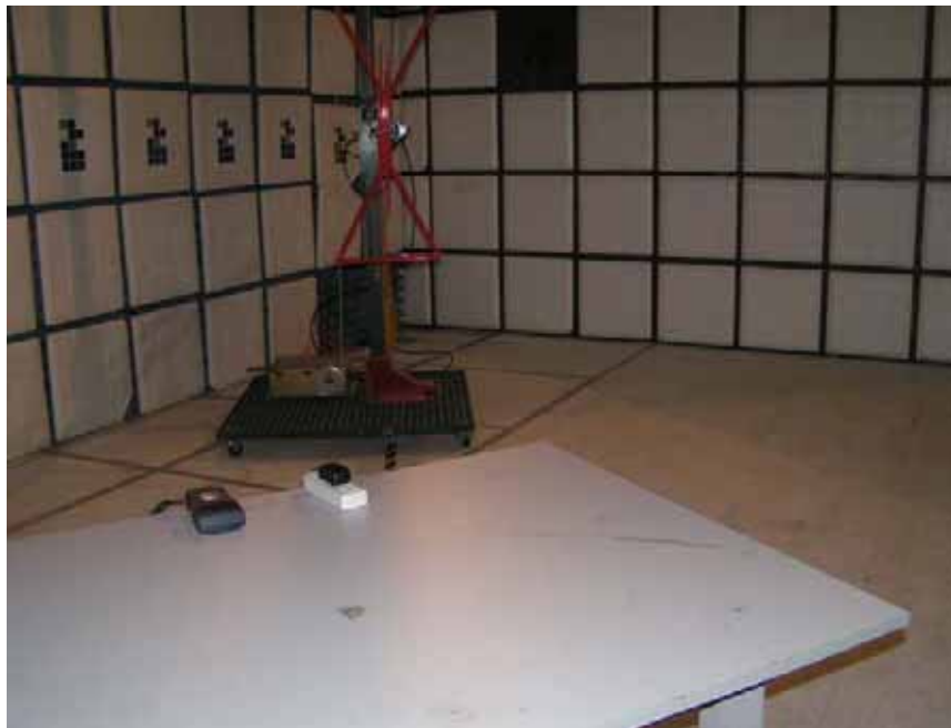
Radiated Emission Test Set-Up – Back View
