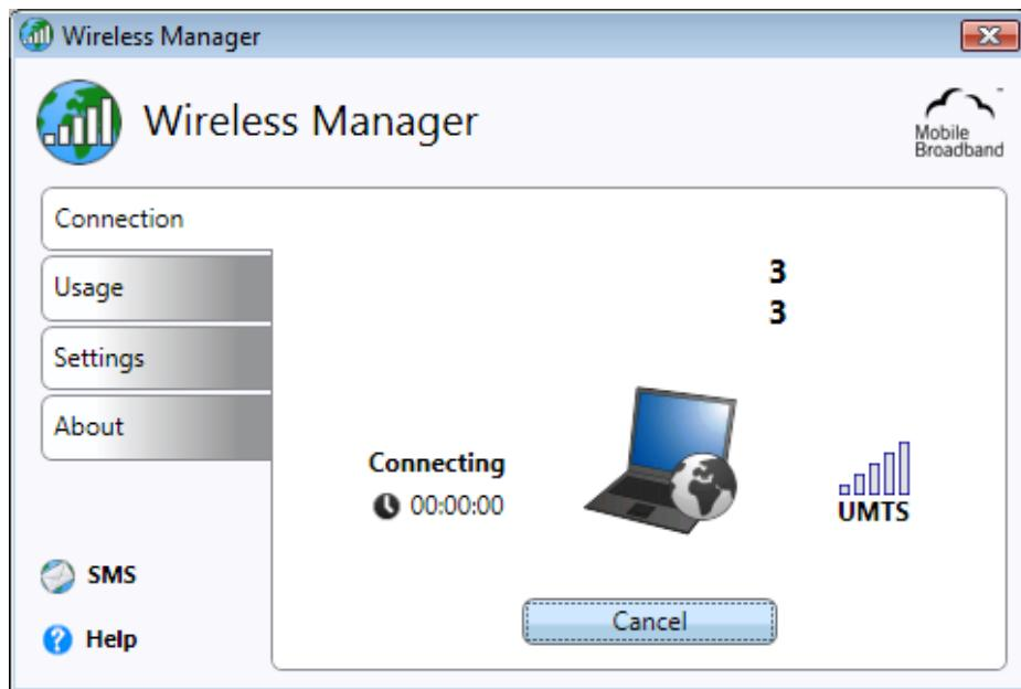
The network operator's and the host device manufacturer's logos can be customized in the application. Connection duration, connection mode, volume of data and an indication of the signal strength are provided in the Wireless Manager window while connection is active. The figures provide an approximate checkpoint of the data volumes. Please note that the information shown here is not guaranteed to match the mobile operator's bill.
