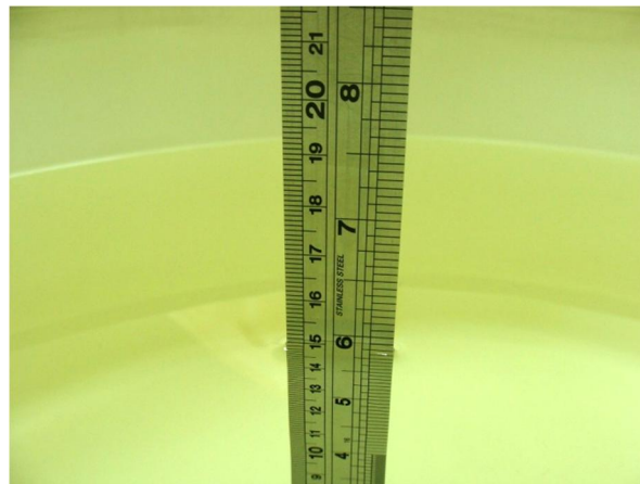
Fig 6.2 Photo of Liquid Height for Body SAR
