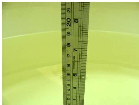
Fig 6.2 Photo of Liquid Height for Body SAR
