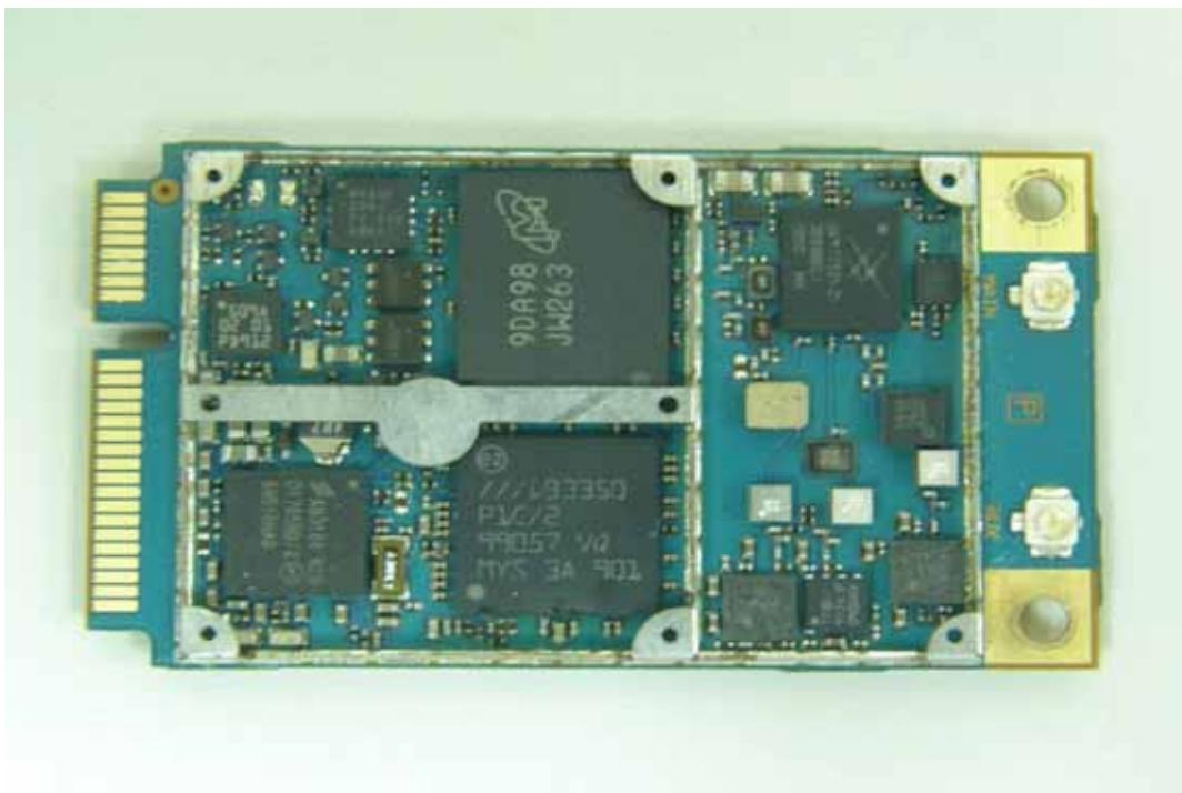
*Internal View of EUT-3 (WWAN Module)*
