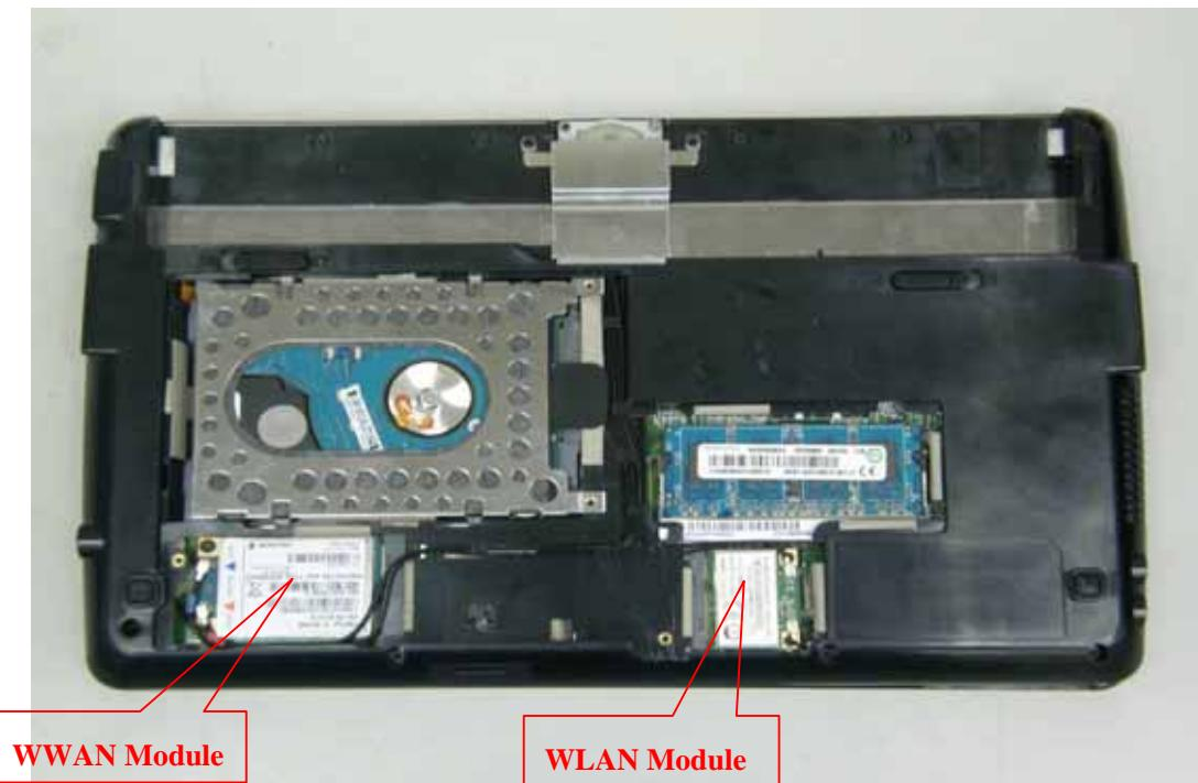
*Internal View of EUT -1 (WWAN Module)*
