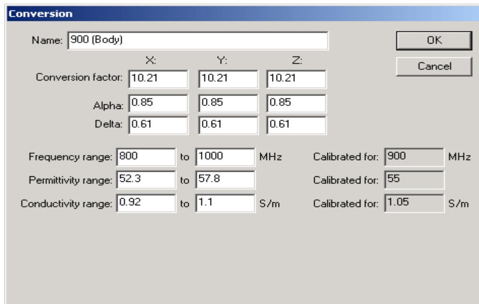
The target permittivity and conductivity at 835 MHz is 55.2 and 0.97 respectively which is within the calibrated range of the probe parameter.
