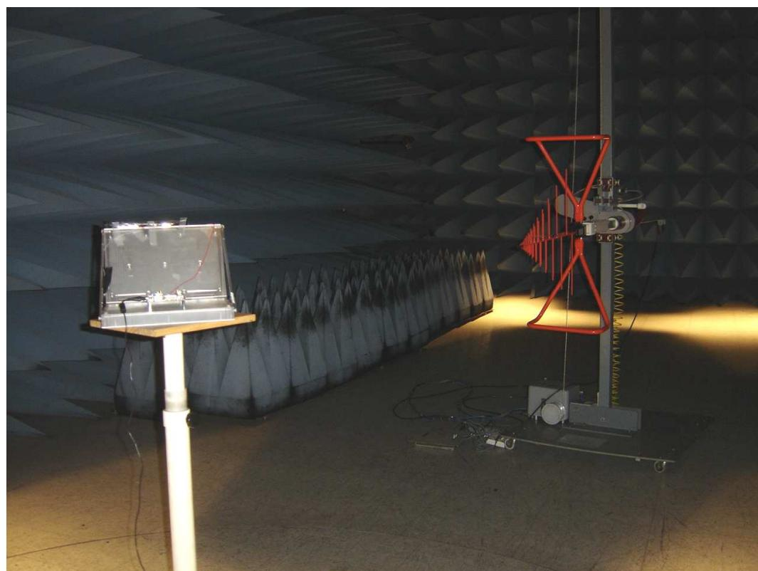
**TEST SET-UP FOR RADIATED MEASUREMENTS ABOVE 1GHz**
