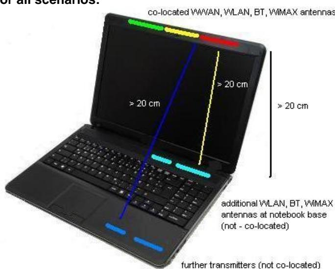
**Important note:** this notebook configuration is an example. Different applications (e.g. M2M) are also possible as long as the same antenna-to-antenna and antenna-to-user distances are respected.
