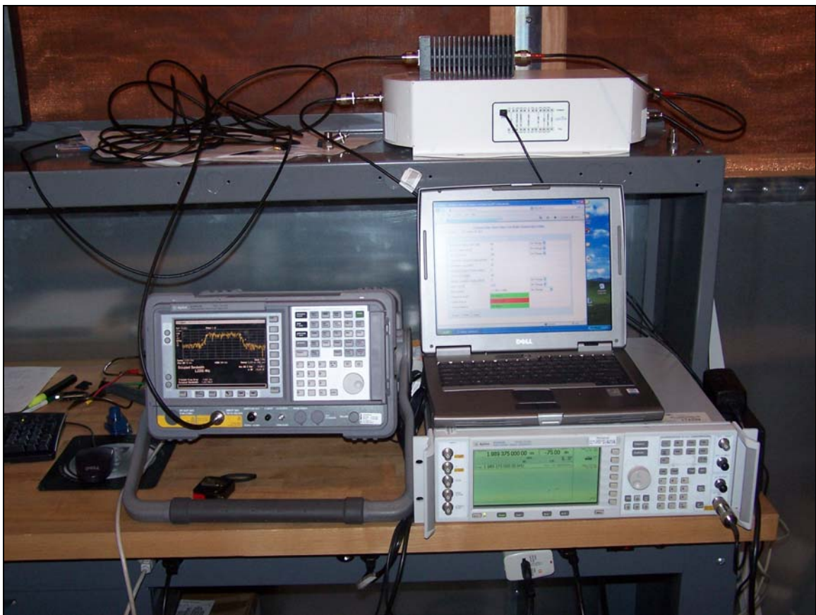
Photograph 2. Conducted Emissions, Test Setup
