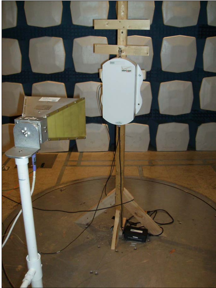
Photograph 4. Radiated Emissions Test Setup
