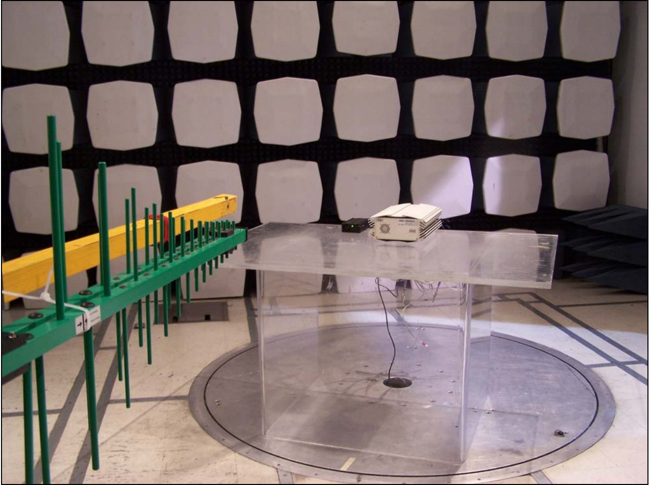
Photograph 2. Radiated Emission Limits Test Setup
