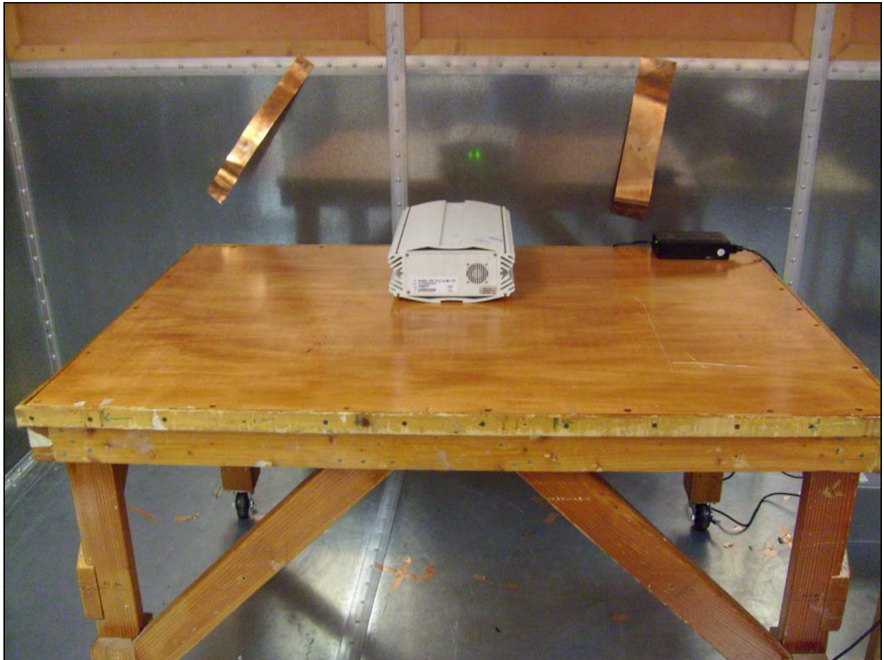
Photograph 1. Conducted Emissions, Test Setup
