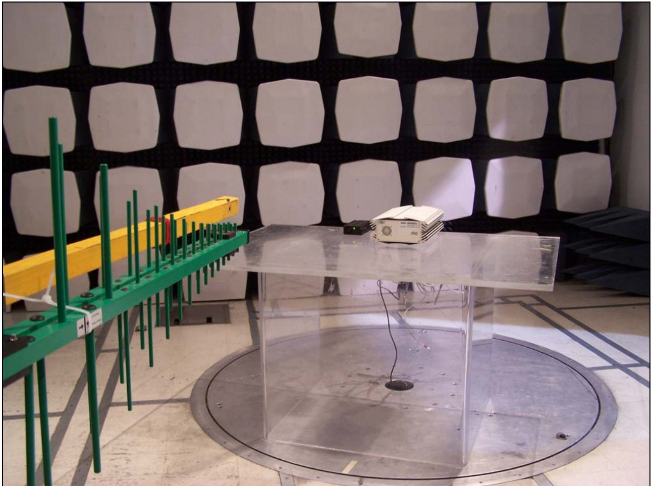
Photograph 2. Radiated Emission Limits Test Setup
