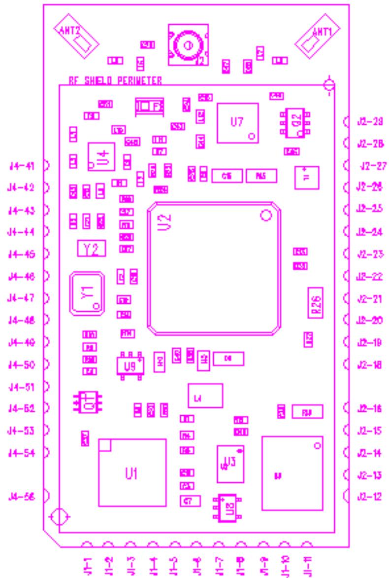
Figure 1. MSR Placement diagram showing pad numbering.
