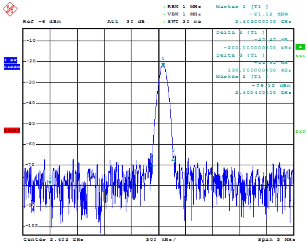
For band frequency 2.400GHz, test level is -79.12dBmW,
