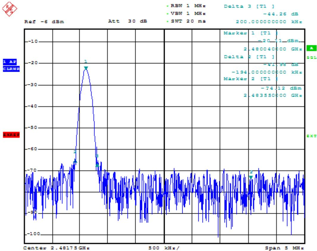
For band frequency 2.4835GHz, test level is -20.11dBmW,
