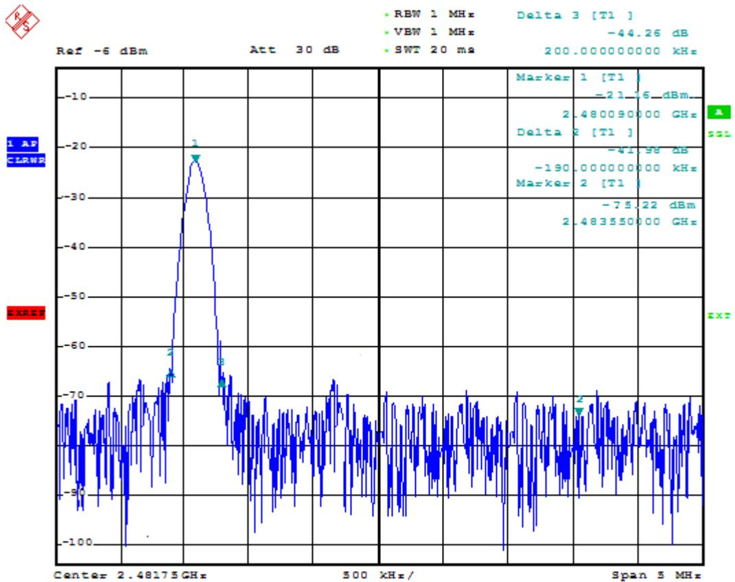
For band frequency 2.4835GHz, test level is -75.22dBmW,
