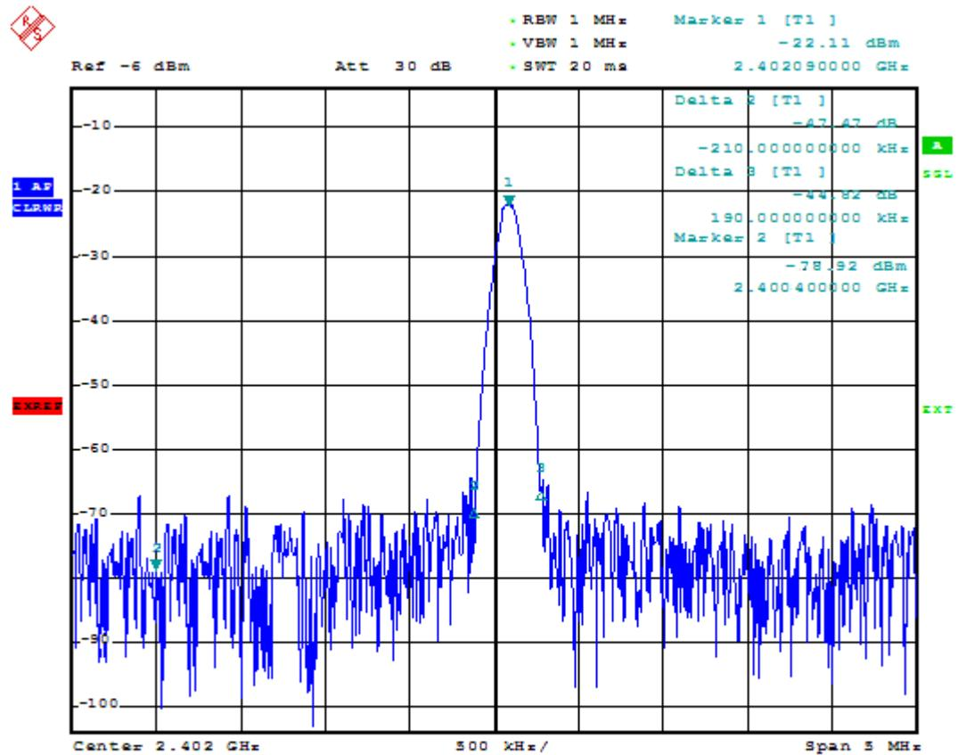
For band frequency 2.400GHz, test level is -78.92dBmW,
