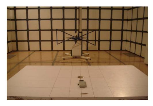
**Radiation Emission Test View For 1GHz-5GHz**
