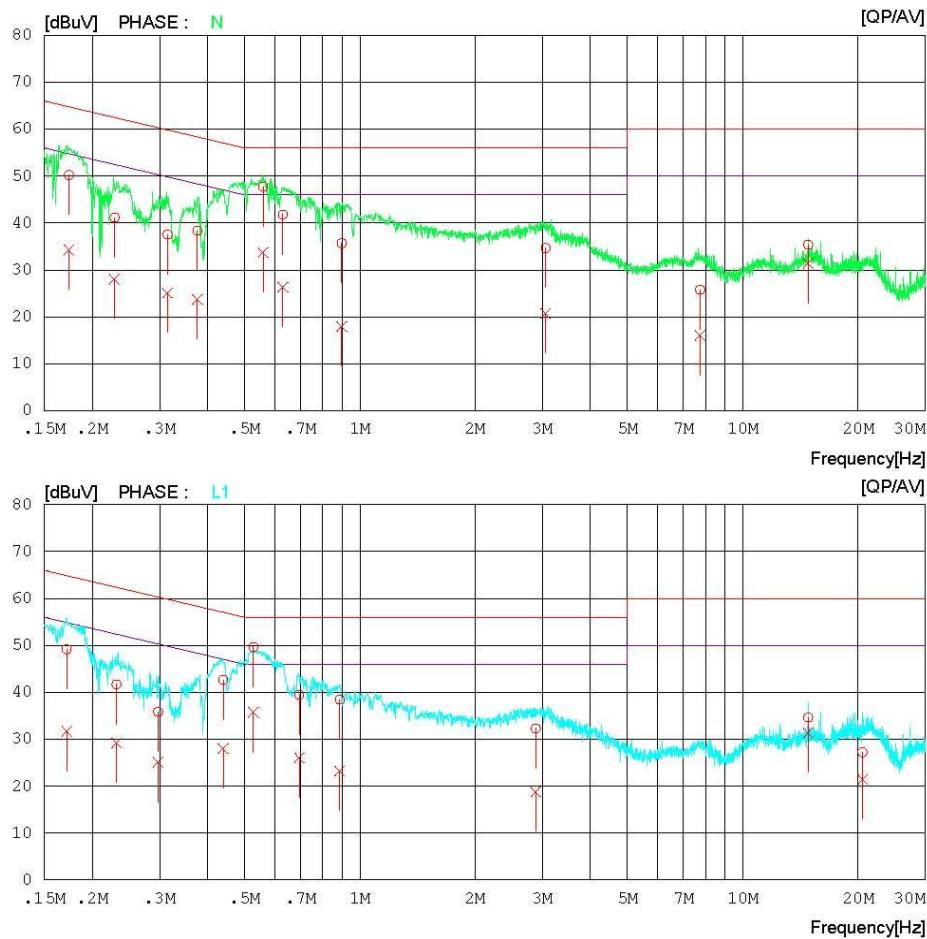
**AC Line Conducted Emissions (List) & Modulation: GFSK****Results of Conducted Emission**Digital EMC
