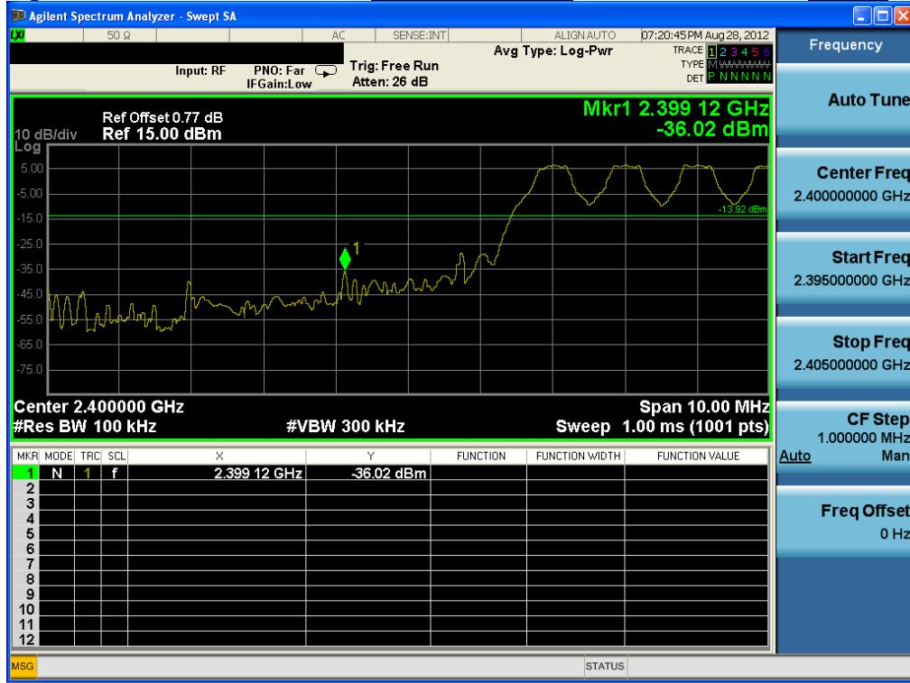
**Conducted Spurious Emissions****Lowest Channel & Modulation: GFSK**
