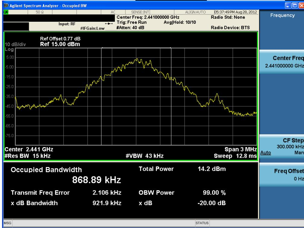
**20dBc Bandwidth****Highest Channel & Modulation: GFSK**
