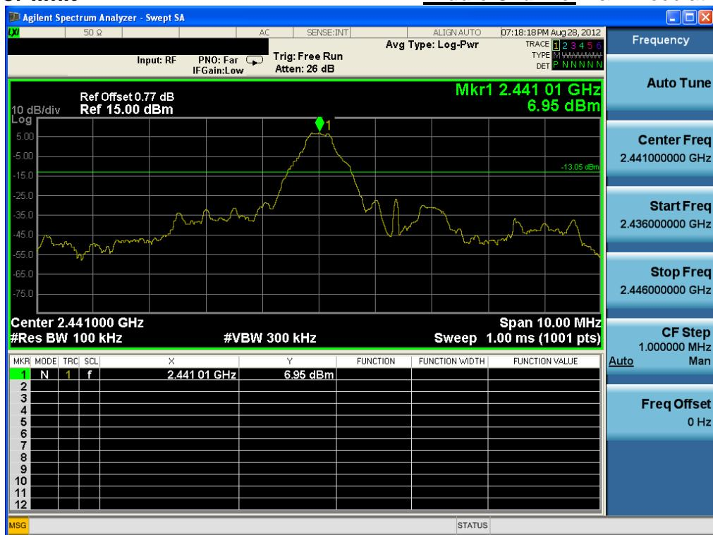
**Conducted Spurious Emissions****Middle Channel** & Modulation: **GFSK**
