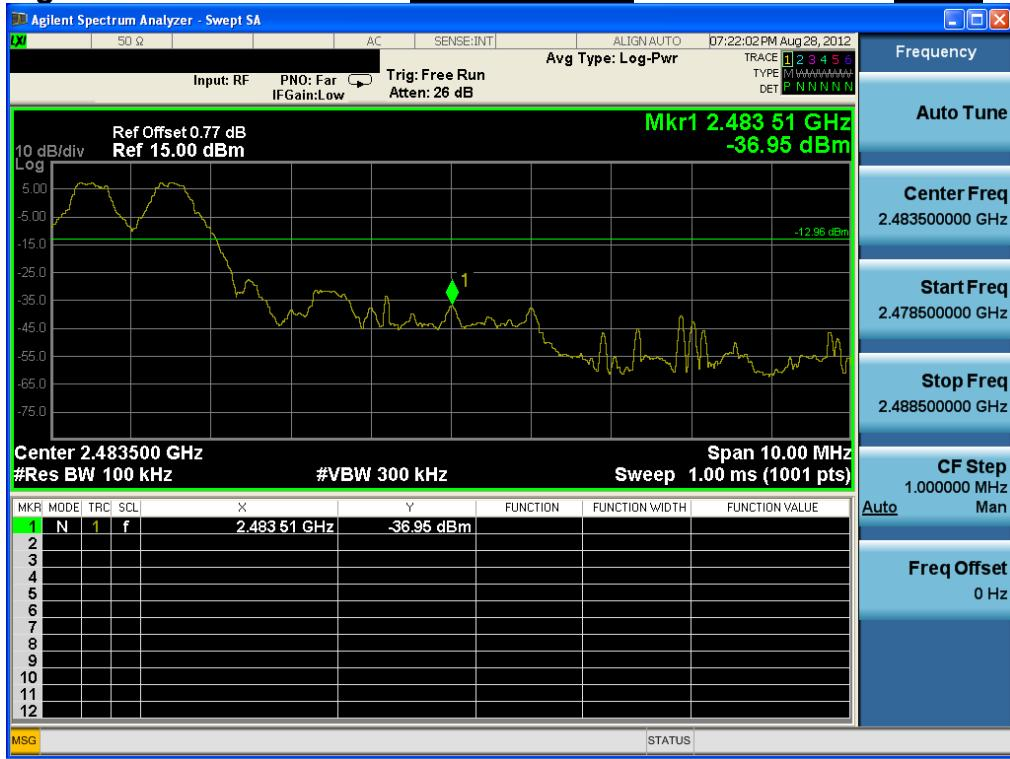
**Conducted Spurious Emissions****Highest Channel & Modulation: GFSK**
