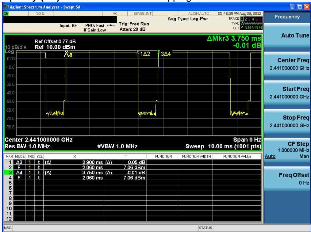
**Time of Occupancy (AFH)****Hopping mode: Enable & Test Case 1**
