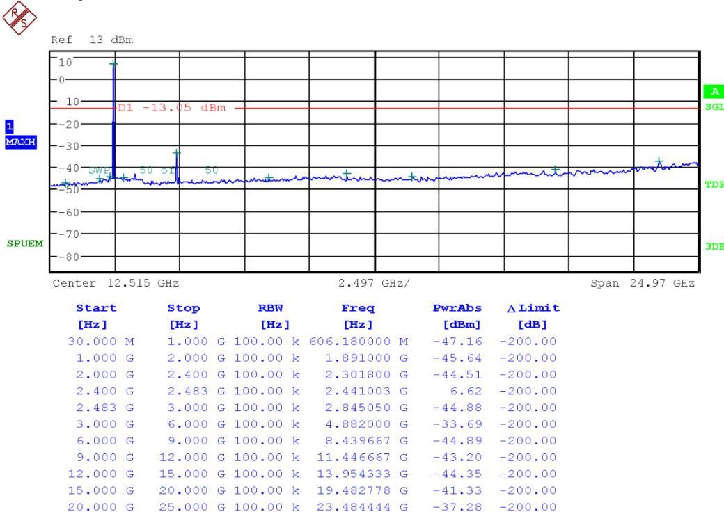
**High Band-edge****Highest Channel & Modulation: GFSK**
