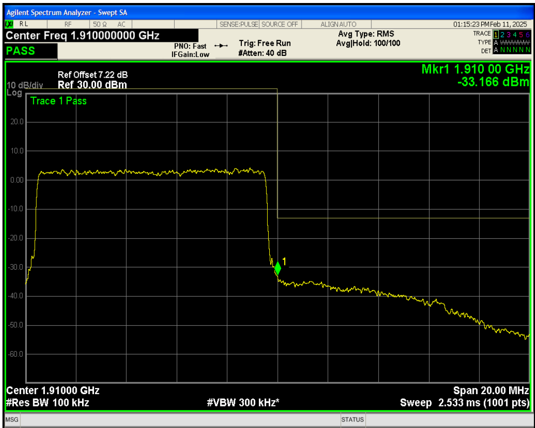
Band2 QPSK BW=15MHz Channel=18675 RB Size=75 Position=#0
