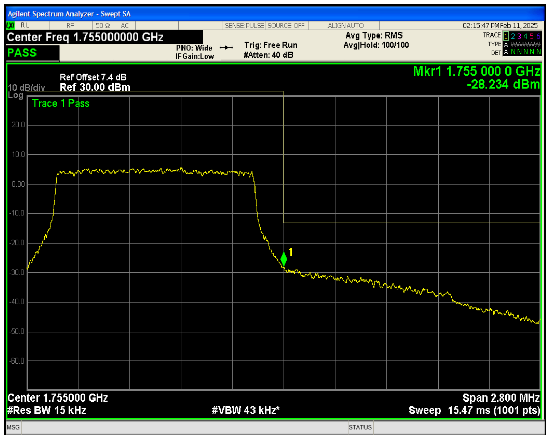
Band4 QPSK BW=3MHz Channel=20385 RB Size=15 Position=#0
