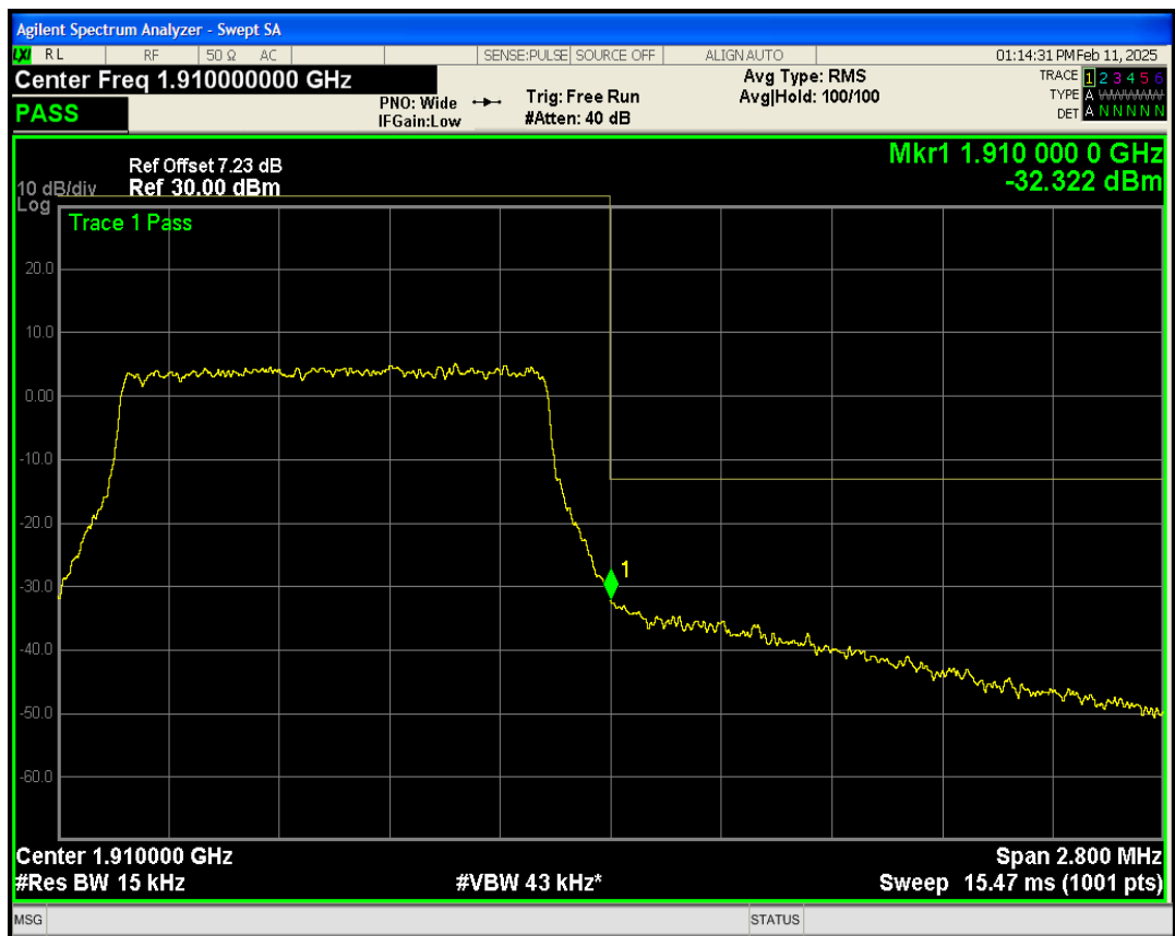
Band2 QPSK BW=3MHz Channel=19185 RB Size=15 Position=#0
