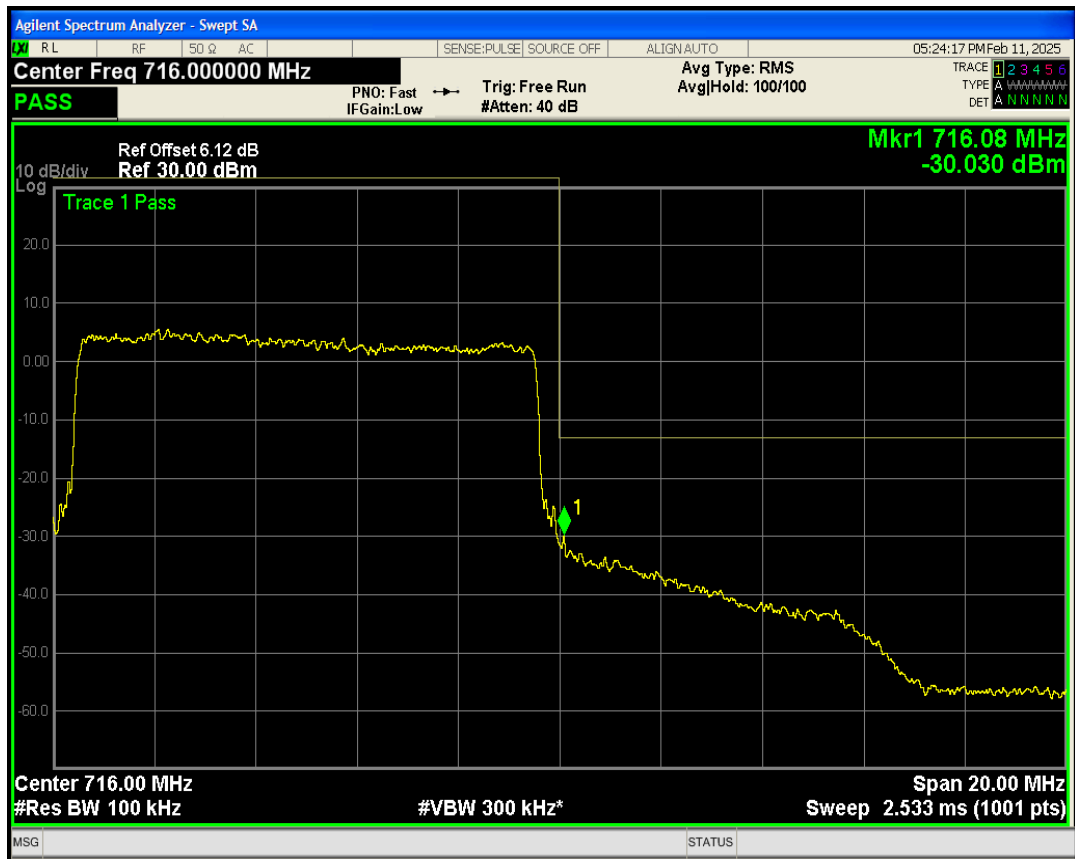
Band2 QPSK BW=1.4MHz Channel=18607 RB Size=6 Position=#0
