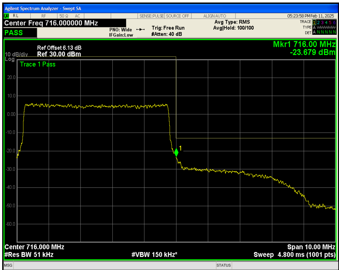
Band17 QPSK BW=10MHz Channel=23780 RB Size=50 Position=#0
