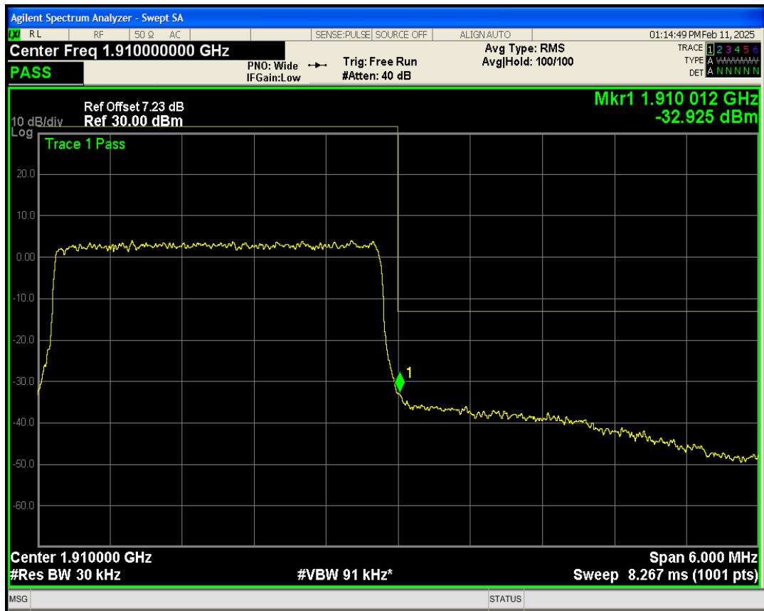
Band2 QPSK BW=5MHz Channel=18625 RB Size=25 Position=#0
