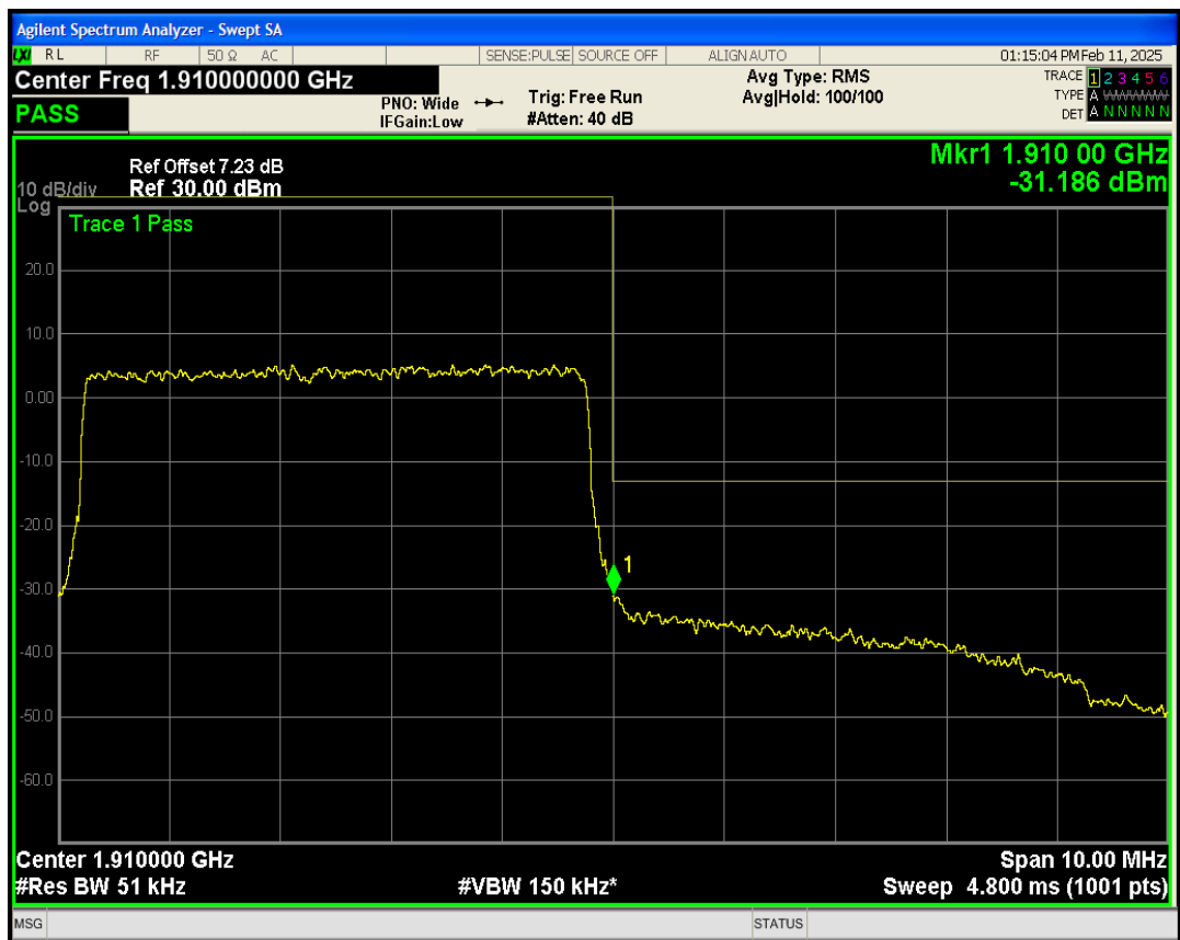
Band2 QAM16 BW=5MHz Channel=19175 RB Size=25 Position=#0
