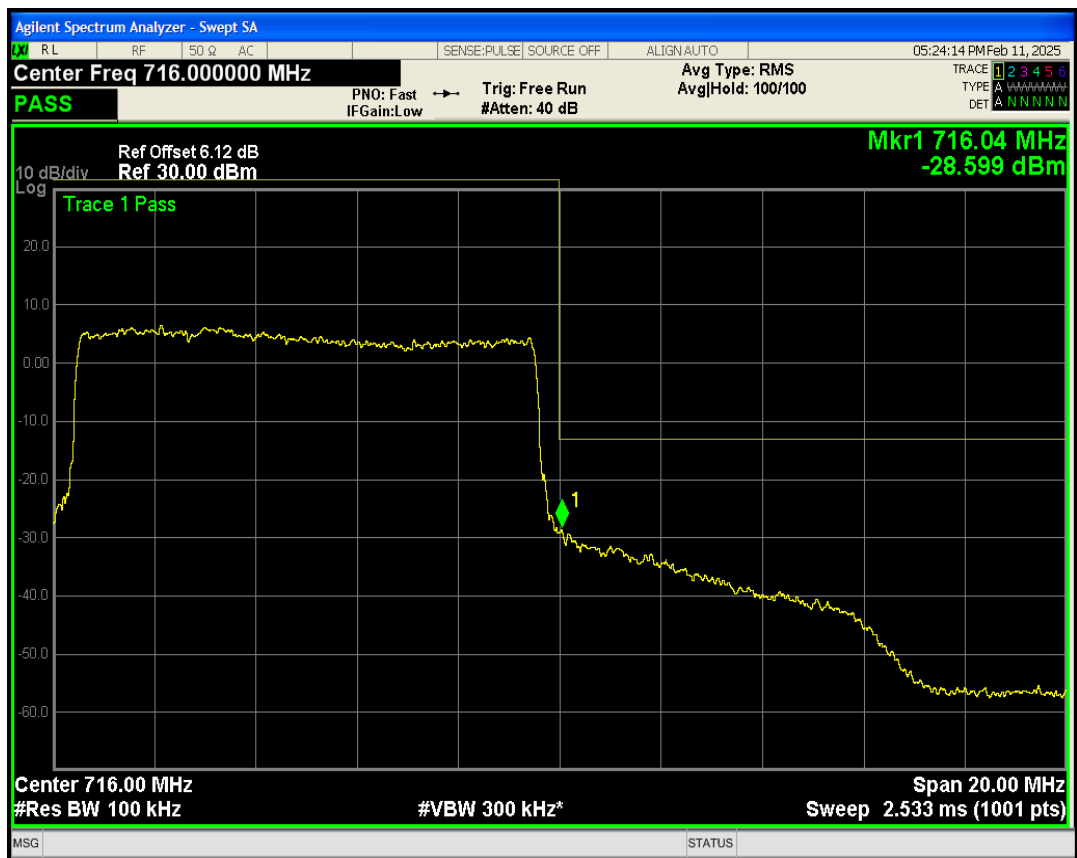
Band17 QAM16 BW=10MHz Channel=23800 RB Size=50 Position=#0
