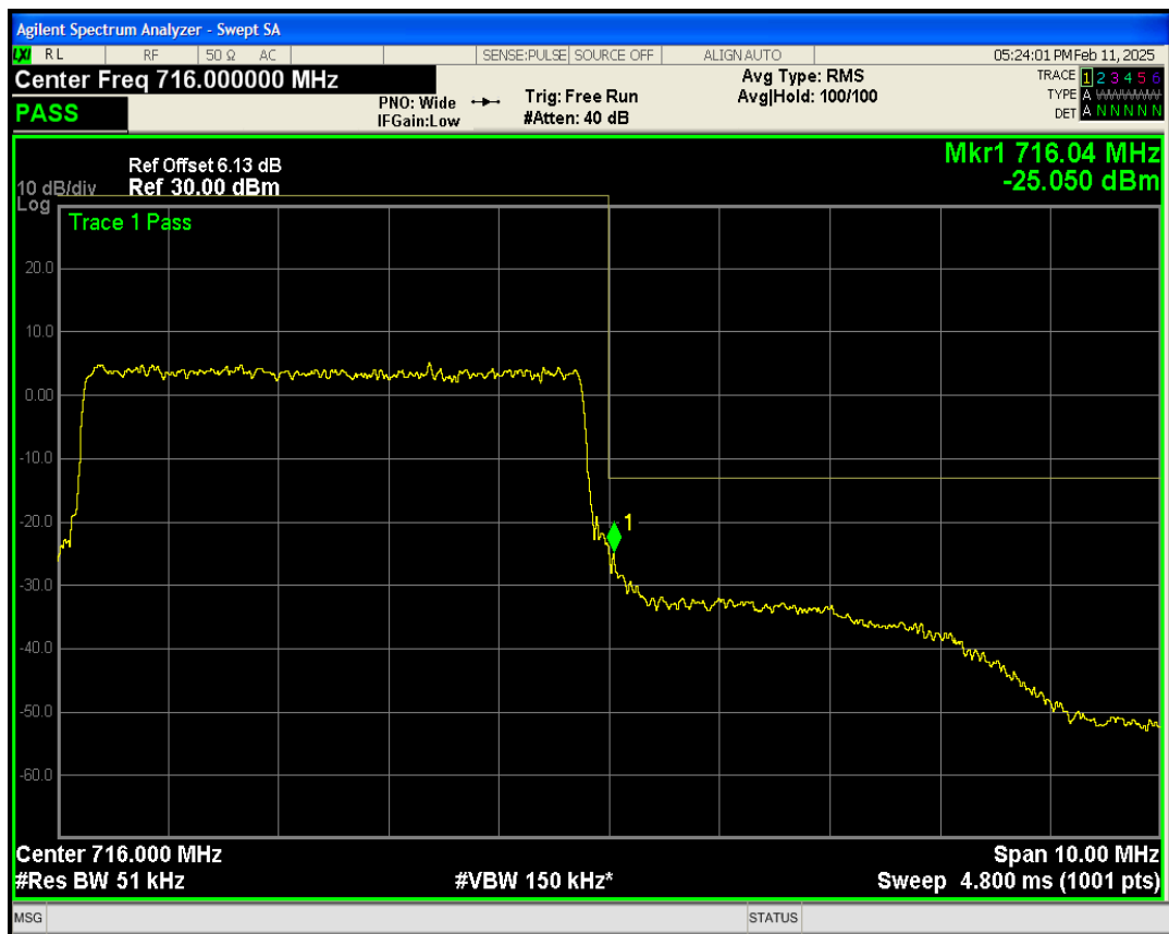
Band17 QAM16 BW=10MHz Channel=23780 RB Size=50 Position=#0
