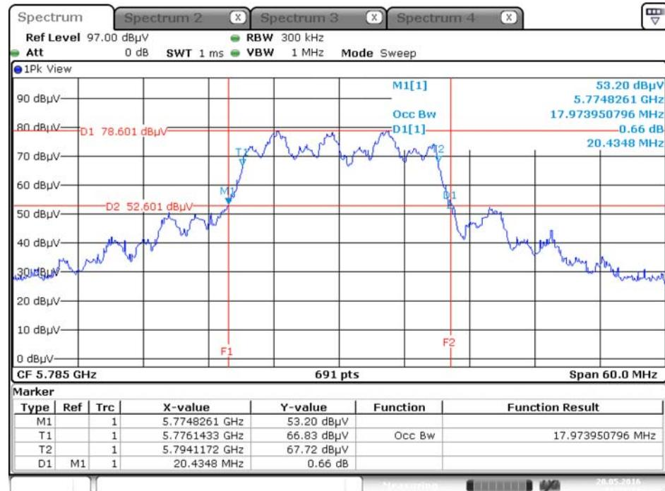
**26dB Bandwidth and 99% Occupied Bandwidth Plot on Configuration IEEE 802.11n MCS0 HT20 / Chain 1 + Chain 2 + Chain 3 / 5825 MHz**
