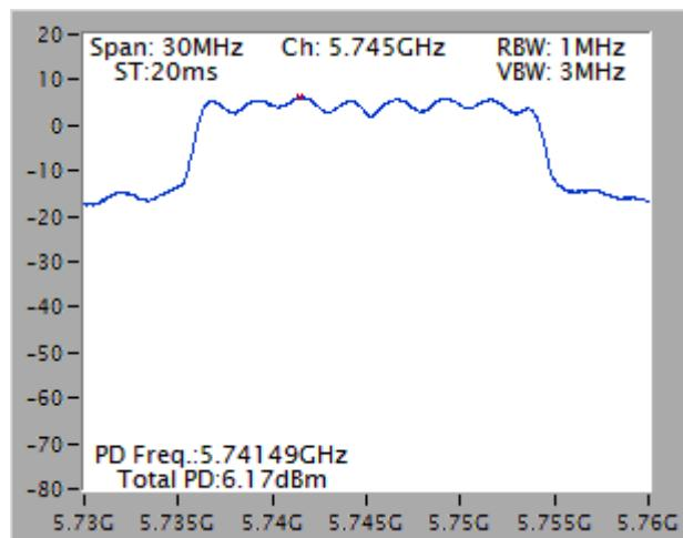
Power Density Plot on Configuration IEEE 802.11n MCS0 HT40 / Chain 1 + Chain 2 + Chain 3 / 5230 MHz
