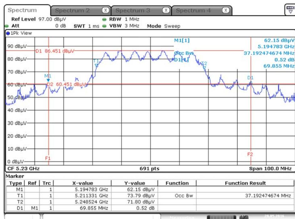
**26dB Bandwidth and 99% Occupied Bandwidth Plot on Configuration IEEE 802.11n MCS0 HT40 / Chain 1 + Chain 2 + Chain 3 / 5755 MHz**
