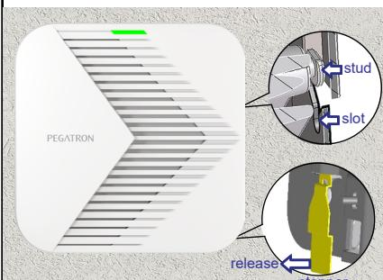
3. Install the security "screw" here to secure the radio unit from sliding out.
