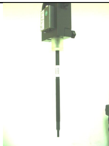
Fig 5.2 Photo of ET3DV6/ET3DV6R
