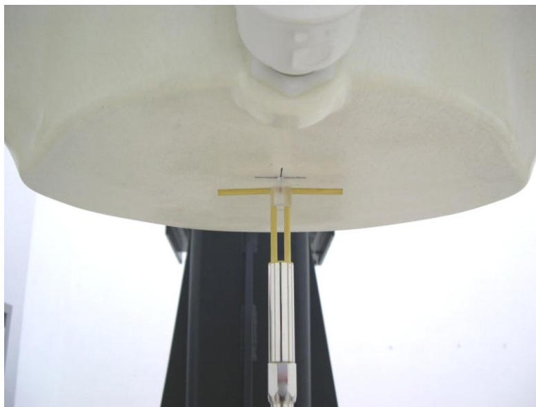
Fig 8.2 Photo of Dipole Setup
