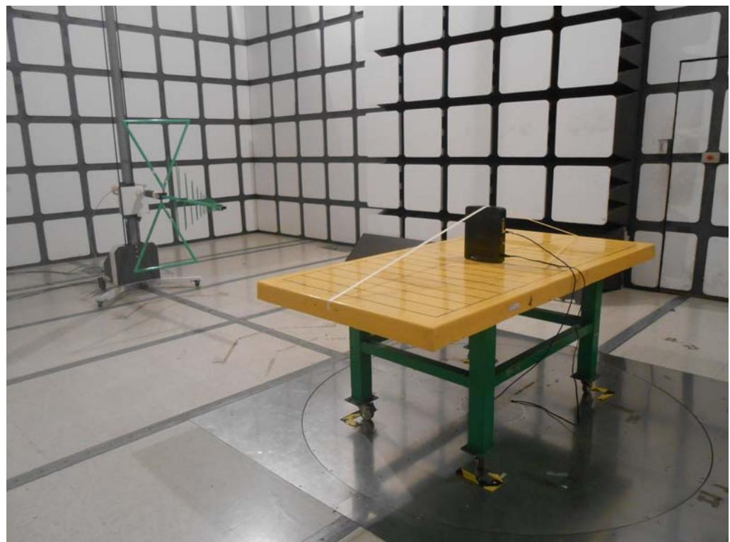
**Test Configuration: Above 1GHz / Mode 1**
