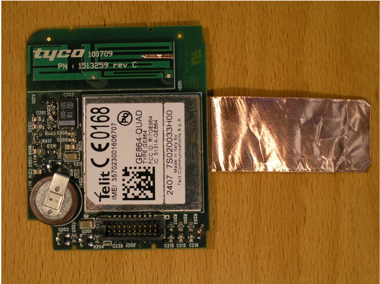
Photograph 4: Equipment under test: Integrated GSM module and internal antenna
