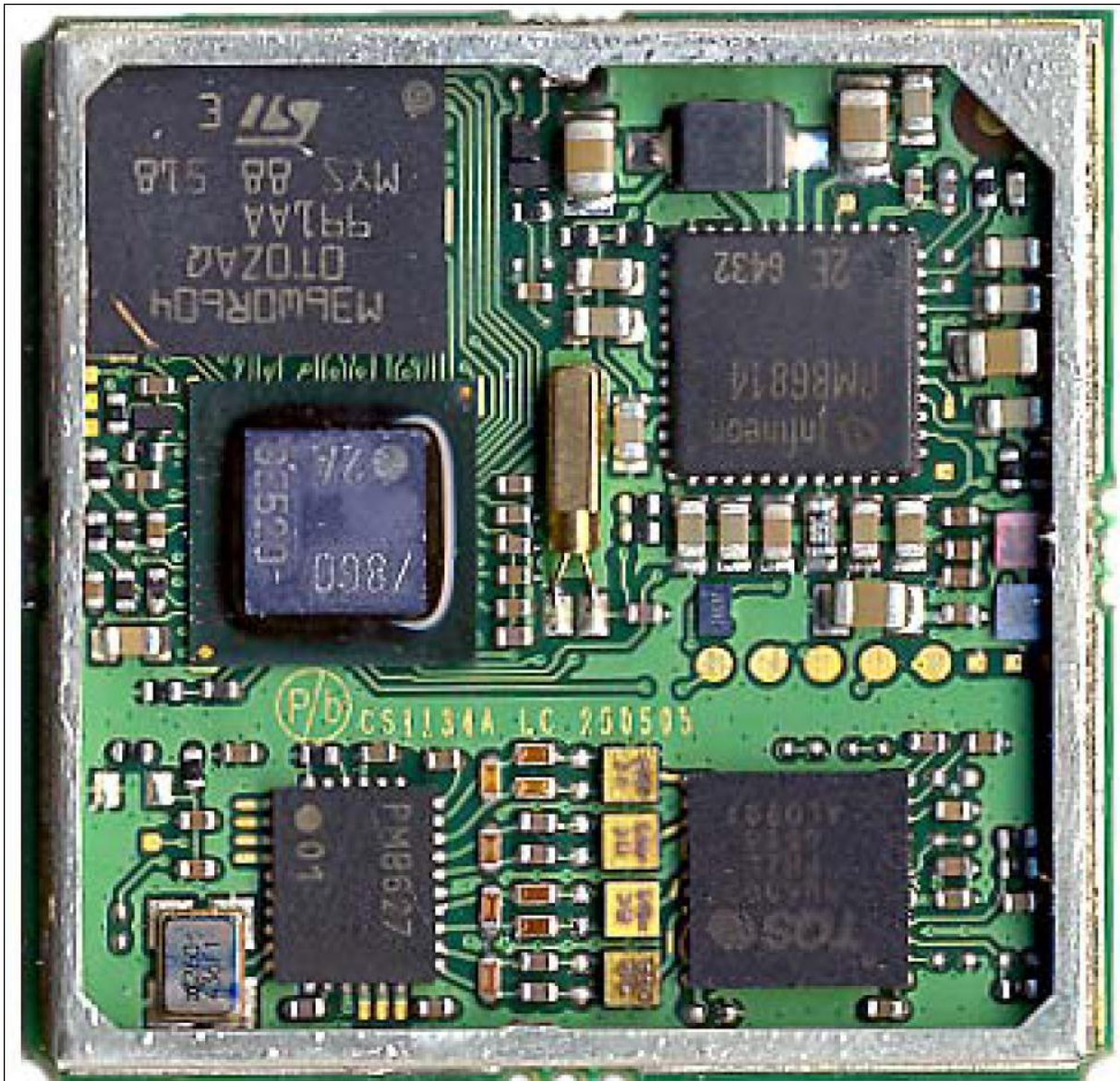
Photograph 5: Equipment under test: Internal Photo of used GSM Module
