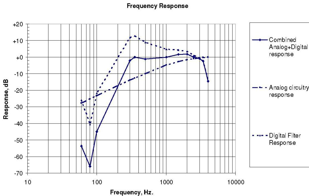
From these curves, we see that the analog filter serves to immediately attenuate the low frequency noise, keeping it from the microphone amps and ADC, reducing saturation and non-linearity problems. The digital filter then serves to restore the frequency response for the main audio passband, while providing a high rate of rolloff to frequencies below 300 Hz, which are known to carry very little audio intelligence for human voice frequencies.
