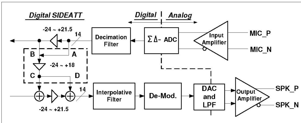
Transmit Audio Input Stage A variable gain amplifier amplifies the signal from MICIN. The analog signal is digitized by a second-order delta-sigma ADC, then converted to 14-bit 8kHz linear PCM data by digital circuit.
