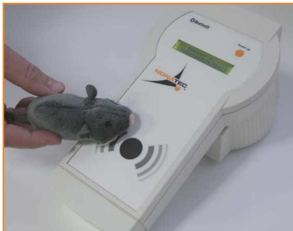
The LAB BENCH reader is designed to allow effortless communication with implanted tags. Information of reading and writing on the **NONATEC** TM tag are displayed on the LCD screen, as well as the unique identification number.
