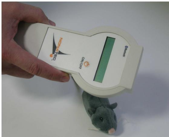
The HAND HELD reader is designed to allow effortless communication with implanted tags. Information of reading and writing on the **NONATEC** TM tag are displayed on the LCD screen, as well as the unique identification number.
