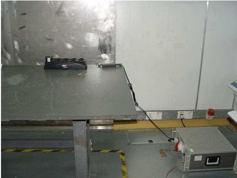
Photograph 2: Set-up for Radiated Emission, below 1GHz, mode A
