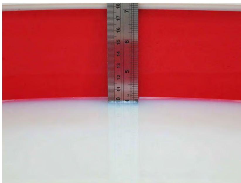
Fig 8.2 Photo of Liquid Height for Body Frequency 5GHz
