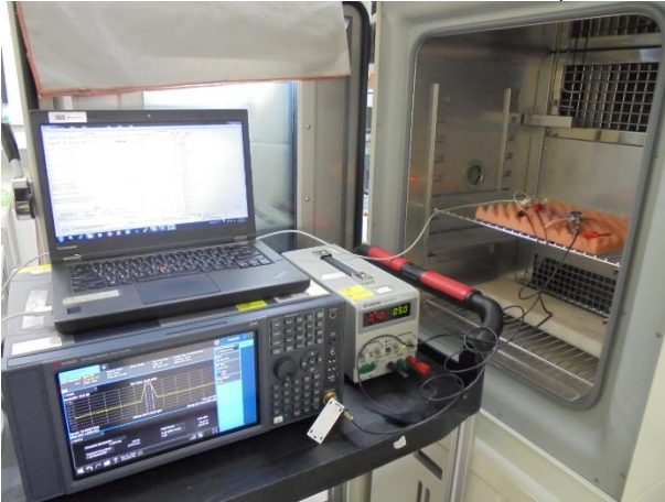
FCC_15_225 / RSS 210_NFC_Radiated_Setup
