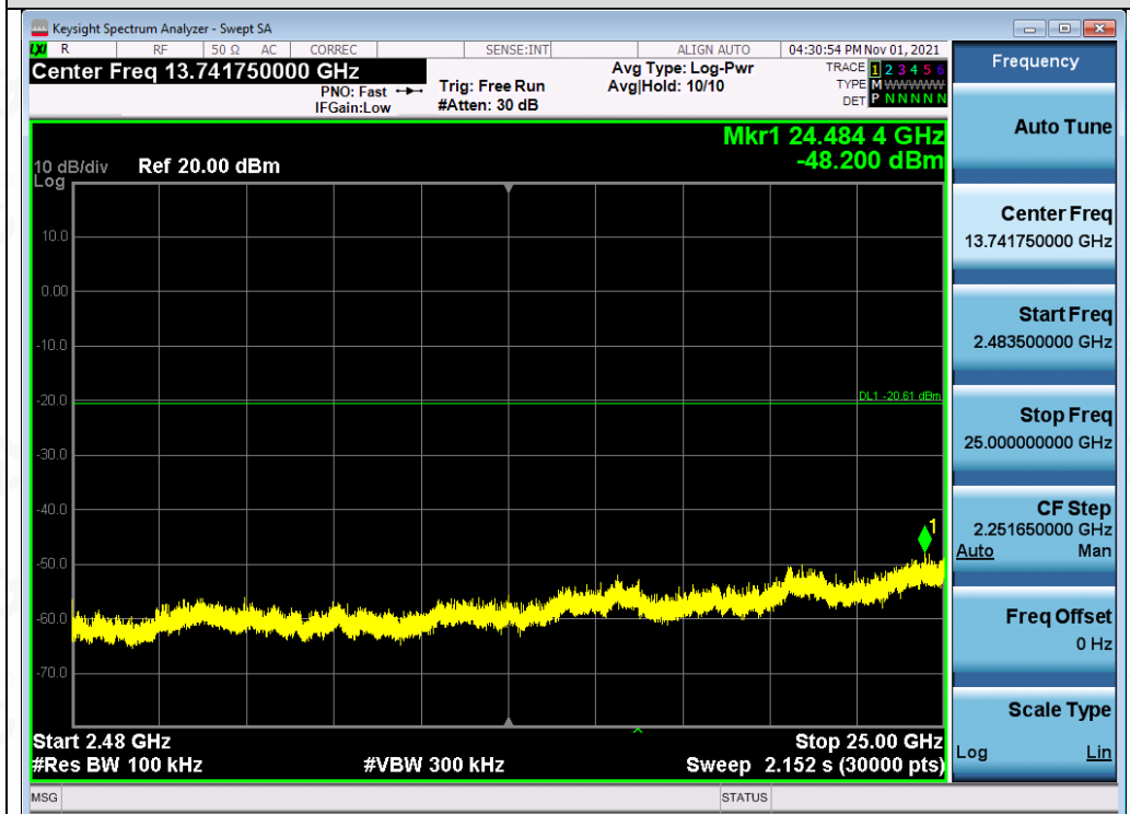
Test_Graph_802.11n20_ANT1_2412_MCS0_Higher Band Emissions
