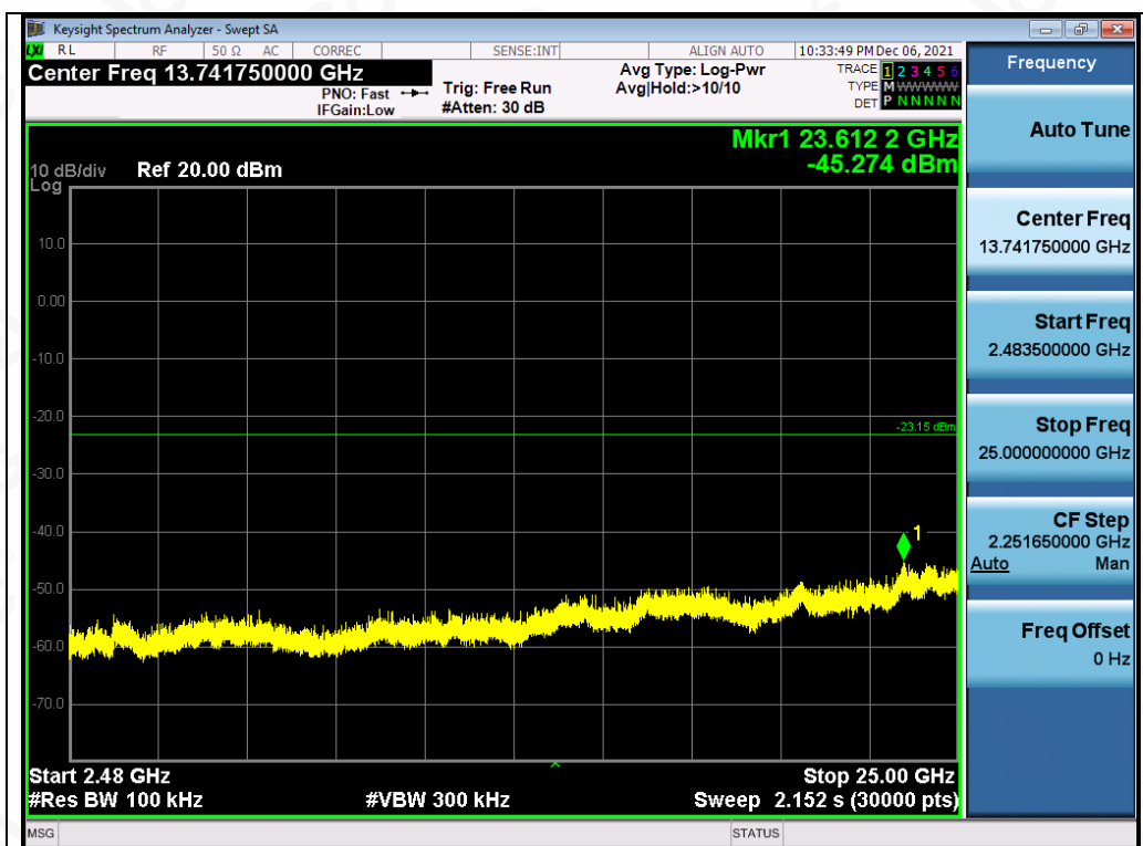
Test_Graph_LE1M_ANT1_2402_1Mbps_Higher Band Emissions
