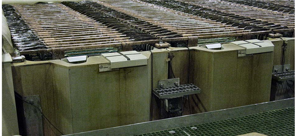
Figure 2. CellSensor Device Installed to an Electrolytic Cell
