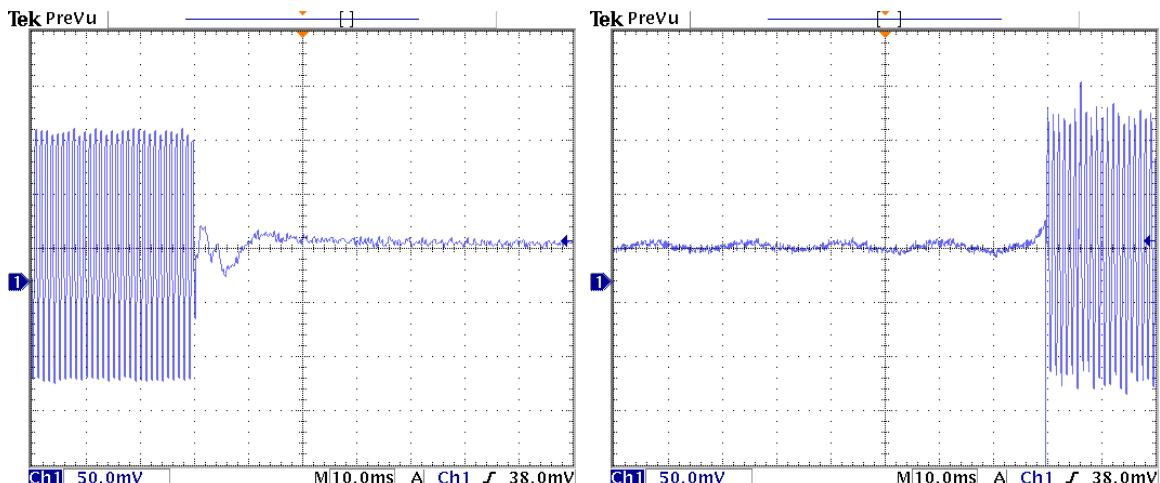
**2. 25 kHz channel spacing****(440.0125MHz 4W)**
