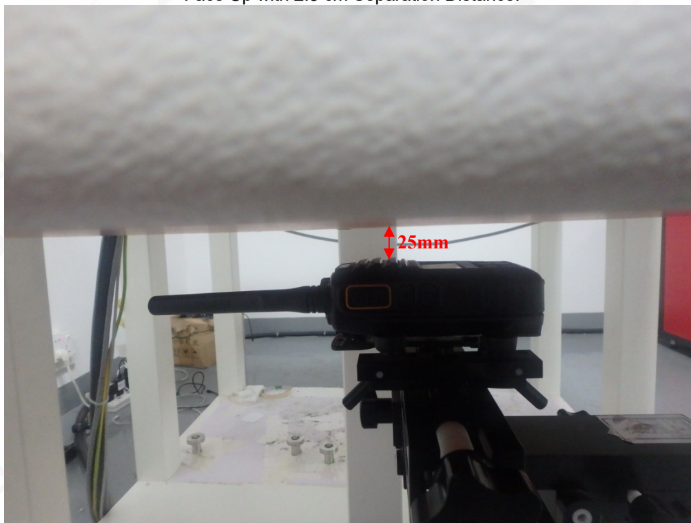
16-Channel Rotary Type Face Up with 2.5 cm Separation Distance.
