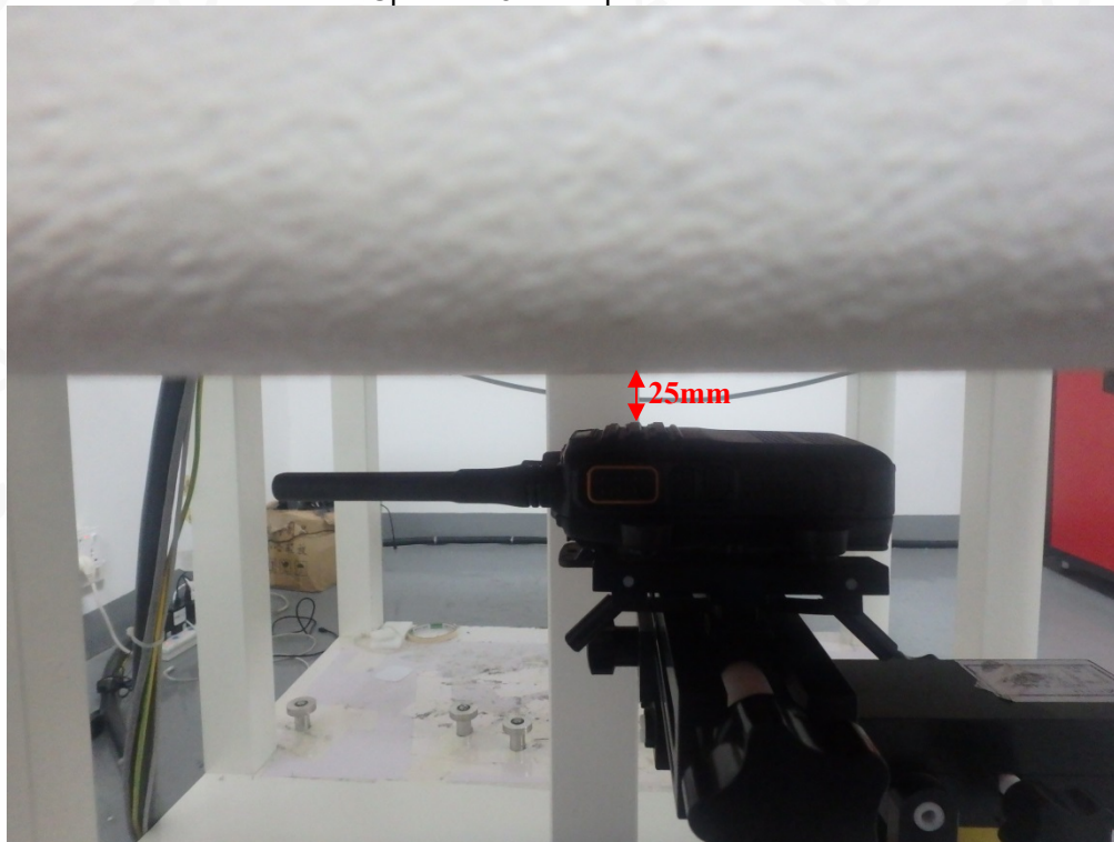
16-Channel Rotary Type Face Up with 2.5 cm Separation Distance.
