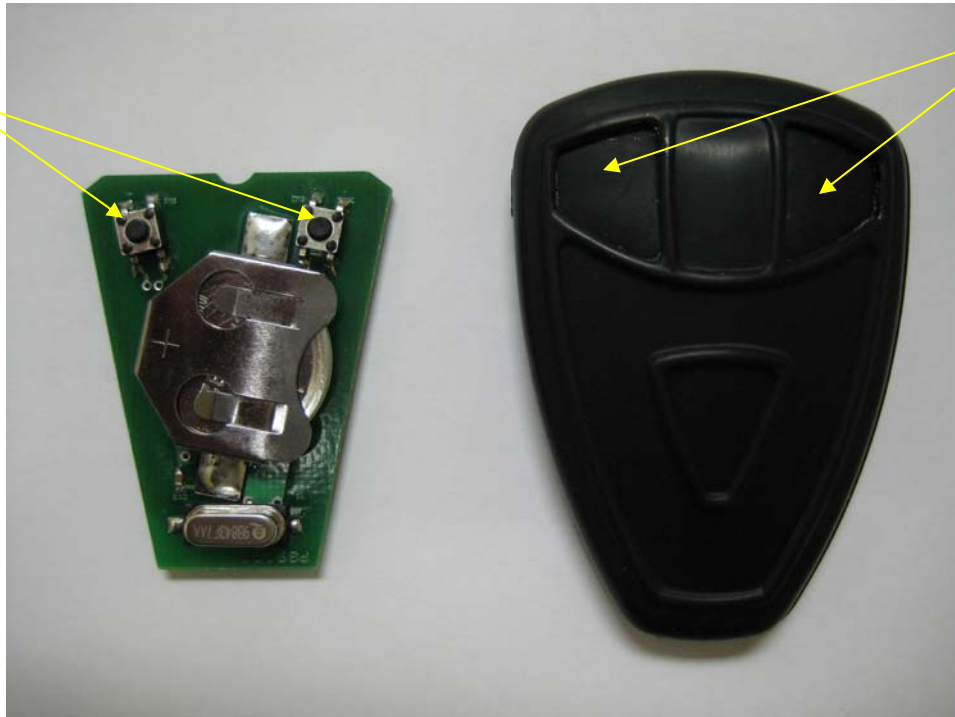
Open, showing two buttons and External view of top-side of Unit Arrows indicate buttons on internal, and external areas of FOB (Issue 3)
