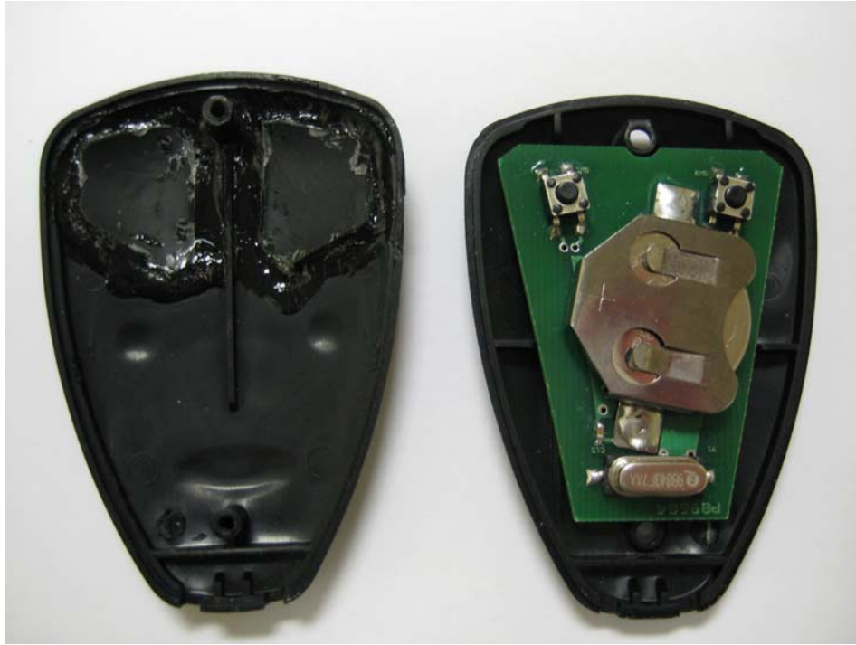
Open, showing two buttons and inside top- side of Unit (Issue 3)
