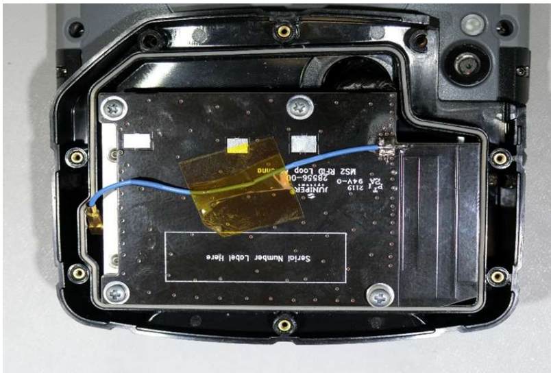
TransCore Module in place
