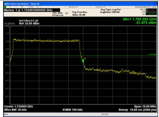
LTE Band IV - High Channel 16QAM-5
